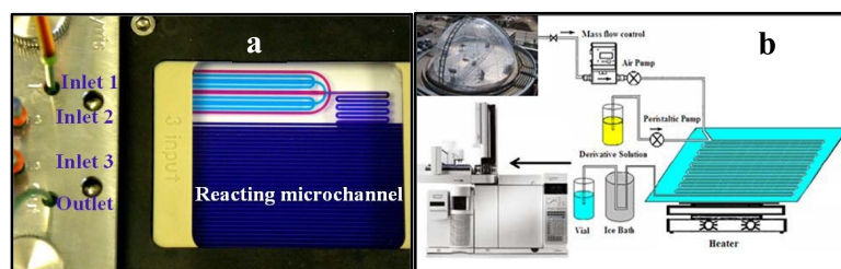
Fig. 1. (a) Basic layout of micro-reactor including three inputs, one output, mixing junctions, and 208 cm reacting microchannel (size: length \times width \times thickness = 90 mm \times 45 mm \times 4.5 mm). (b) Schematics of the microfluidic lab-on-chip derivatization system. Derivative solution was collected directly from micro-reactor and ready to GC-MS analysis.
