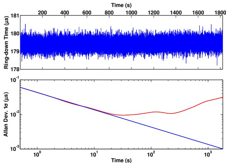
**Fig. 7.** Top: sample ring-down data when the optical cavity was purged with ultra-zero air. Bottom: modified Allan Deviation of the ring-down data (red solid line) as compared to the idealized data without drift, i.e.  $t^{-1/2}$  dependence (blue dashed line). The average rate at which ring downs are acquired is  $\sim 20$  Hz, however, it is not constant, as the computer simply triggers whenever a resonance is detected.
