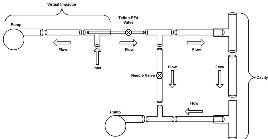
**Fig. 5.** Schematic diagram of the HCl sensor gas flow system. The virtual impactor, indicated on the left, serves to remove large particles from the main sampling flow. The optical cavity is indicated on the right.
