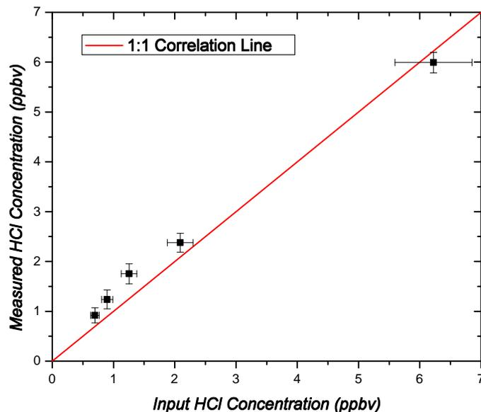
**Fig. 8.** HCl concentration measurements averaged for 10 min as compared to the concentration supplied to the inlet from the calibration system. The solid line shows the expected 1 : 1 correlation between the measured and input values.
