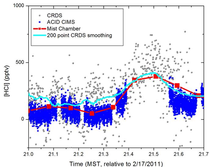
**Fig. 10.** HCl concentration values recorded by the CRDS, ACID CIMS, and mist chamber instruments during the NACHTT campaign.
