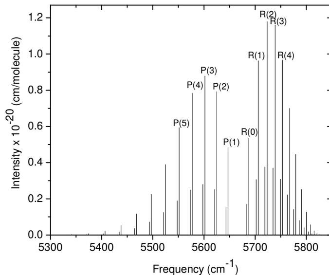
**Fig. 1.** Linestrengths of rotational lines of the 2-0 vibrational absorption band of  $\text{H}^{35}\text{Cl}$  and  $\text{H}^{37}\text{Cl}$  from HITRAN. The CRDS sensor uses the R(3) line of  $\text{H}^{35}\text{Cl}$  at  $5739.26\text{ cm}^{-1}$ .
