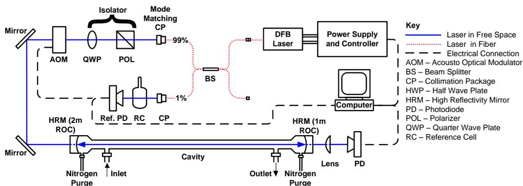
**Fig. 3.** Schematic of the optical components and data acquisition systems of the HCl sensor.
