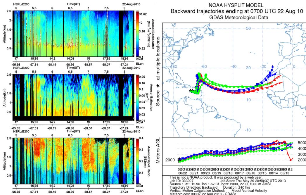
**Fig. 6.** HSRL-1 measurements (left three panels) of aerosol backscatter coefficient, aerosol extinction coefficient and aerosol depolarization ratio,  $\delta$ , on 22 August 2010 in the Caribbean Sea. High values of depolarization indicate a layer of transported Saharan dust, which is mixing with the marine boundary layer. On the right is a set of NOAA HYSPLIT back-trajectories ending within the observed dust layer; the trajectories lead back to Saharan Africa.
