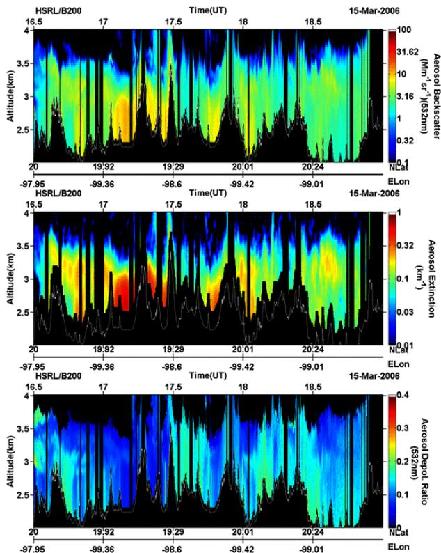
**Fig. 2.** HSRL-1 measurements of the aerosol backscattering coefficient at 532 nm (top), the aerosol extinction coefficient at 532 nm (middle) and the aerosol depolarization ratio,  $\delta$ , at 532 nm (bottom) are shown for a flight over Mexico City and surrounding regions on 15 March 2006 during the MILAGRO campaign. Black vertical lines indicate no data, usually due to shuttering the laser during aircraft turns or filtering data that is attenuated by clouds.
