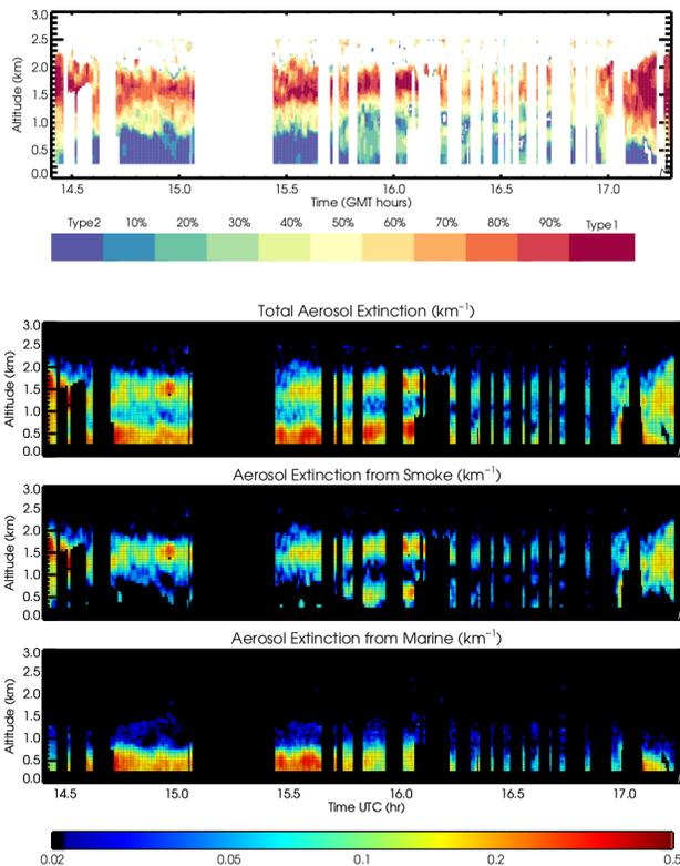
**Fig. 11.** Top shows mixing ratio (percentage of 532-nm backscatter due to smoke) for the mixtures of marine and smoke aerosol observed by HSRL-1 on 28 March 2006 in the Gulf of Mexico. The mixing ratio is inferred from the measurements and Eqs. (30)–(32) as described in the text. Blue indicates marine and red is smoke. Bottom three panels show the partition of aerosol extinction at 532 nm into separate contributions by marine and smoke.
