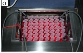
**Fig. 1. (a)** Cold bath set-up, ready for analysis with camera recording from above; **(b)** LED array and polycarbonate plate holding 52 sample tubes; **(c)** detail of tubes and  $Pt_{1000}$  sensors in the corners of the grid inside the cooling bath.
