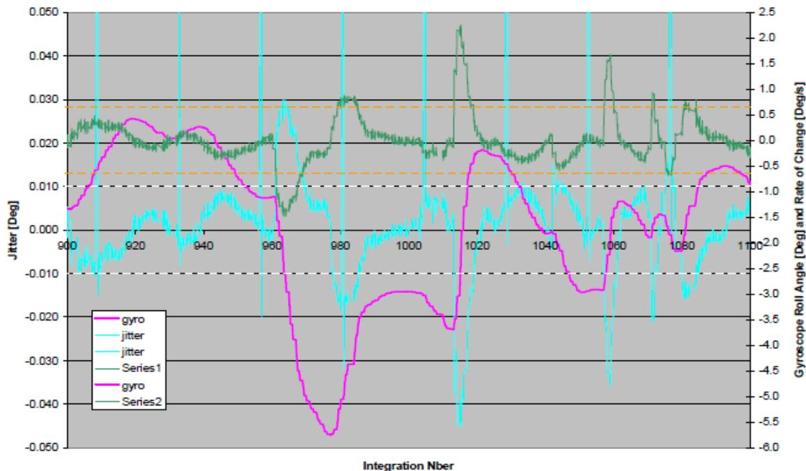
**Figure 4 Reply:** Analysis of pointing precision during a flight jitter is contained within the required  $\pm 0.01$  deg range (highlighted by the white dashed lines) when the absolute roll angle rate of change is contained within the  $\pm 0.63$  deg/s design range (highlighted by the orange dashed lines).
