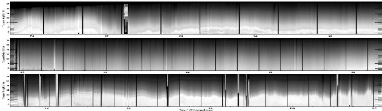
**Figure 2 Reply:** Another indication that the pointing knowledge is good is this reconstruction of individual frames from the optical cloud monitor. Using our roll angle data, we have collated the individual pictures of the camera that is mounted fix to the airframe, and obtain a smooth cloud top surface.
