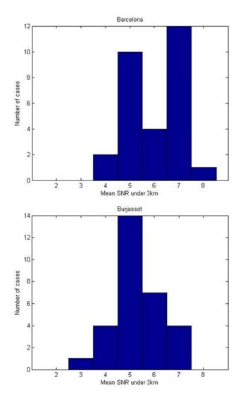
We can see that in most of the cases, a SNR greater than 4.5 is obtained. However, although lower values of SNR have been found, we can use the estimated uncertainty to see how reliable are the extinction profiles found for each case.
