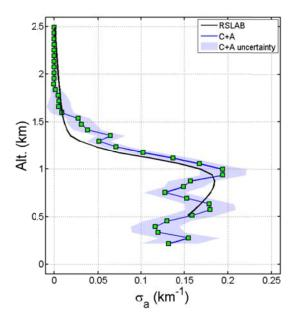
we can also see oscillations within the boundary layer. However, these oscillations have bigger amplitude than in case a, and also a larger spatial scale than the resolution of the profile. This means that in addition to noise, the C+A results at these altitudes are also affected by the spatial aerosol variability, which does not correspond to aerosol time variability over the RSLab, at least between 0.5 and 1 km where a smooth and continuous decrease in  $\sigma^a$  is seen.
