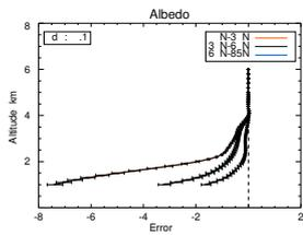
**Fig. 13.** Average error profiles from 10–60 km for three different latitude bands (Northern Hemisphere), i.e., tropics (red diamond), mid latitude (solid line), and polar region (blue cross) and for the following parameters (a) aerosol, (b) albedo, and (c) temperature.
