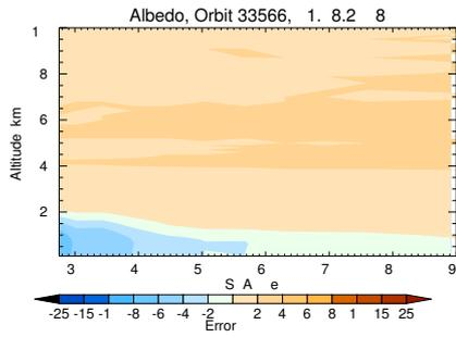
**Fig. 7. (a)** Contour plot of the ozone retrieval error as a function of solar zenith angle and altitude for an albedo perturbation of 0.1 and for the Orbit 33566.
