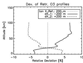
**Fig. 9.** Similar to Fig. 6 but for the following parameters: **(a)** pressure, **(b)** tangent height, and **(c)** temperature sensitivity of  $O_3$  absorption cross section (T-ozone). The viewing geometry is taken from SCIAMACHY orbit 33566 (1 August 2008) at geolocation of  $70^\circ$  N and  $165^\circ$  E, with azimuth angle of SAA:  $29^\circ$ , solar zenith angle of SZA:  $52^\circ$ .
