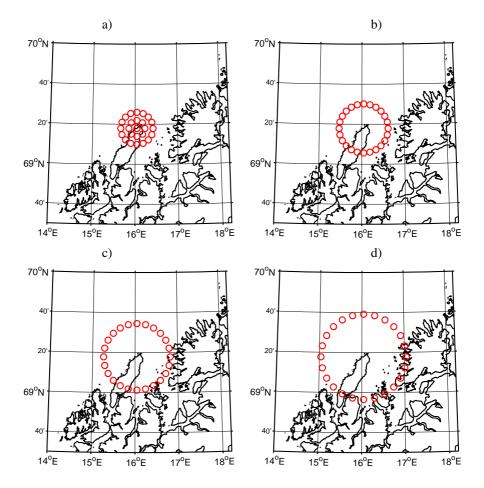
**Fig. 2.** The multi-beam sequence is conducted using 4 experiments with 25 beams each. The black contour lines indicate the Northern Norwegian coast line. The red circles represent the beam positions assuming a 3.6° beam width at 84 km.. **The labels a,b,c,d correspond to the experiments meso006a25, meso006b25,meso006c25 and meso006d25 summarized in Tab. 1.**
