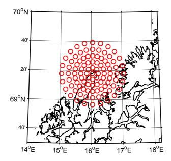
**Fig. 1.** Beam position of MAARSY scanning experiment during summer 2011. The black contour lines indicate the Northern Norwegian coast line. The red circles represent the beam positions assuming a  $3.6^{\circ}$  beam width at  $84 \,\mathrm{km}$ .
