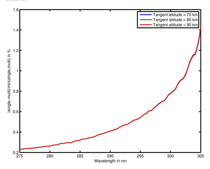
The following figure shows a comparison of the 3 different scenarios. Even for the worst case scenario the differences between multiple and single scattering at 285 nm are less than 1% and thus multiple scattering is neglected.
