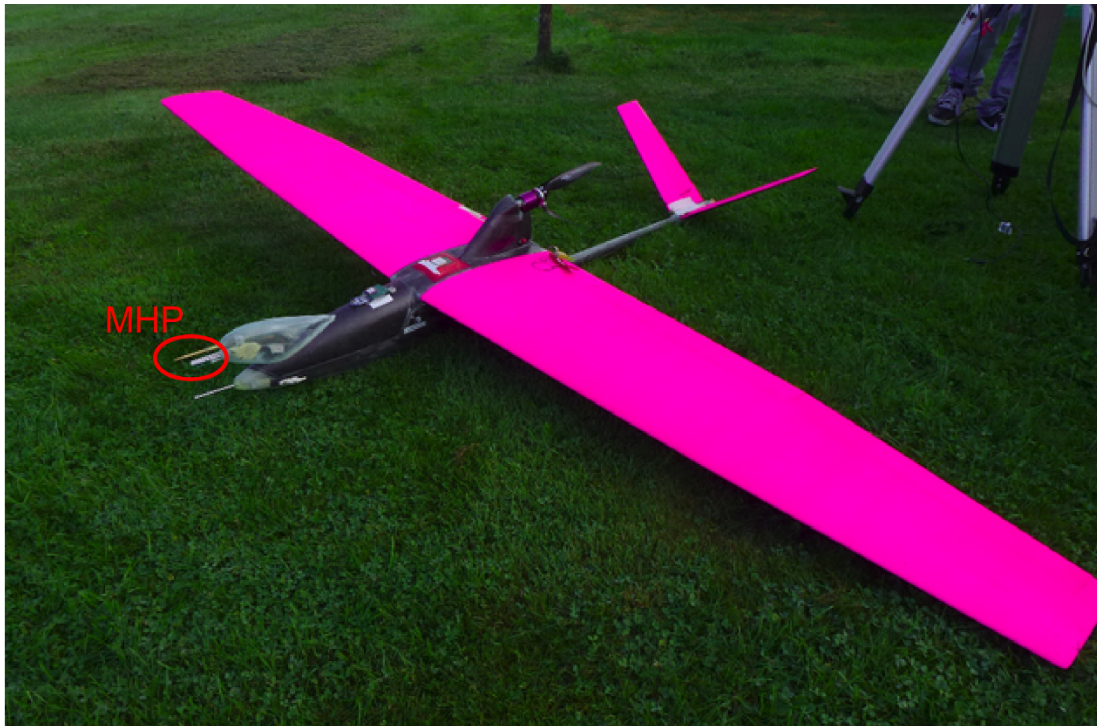
Fig. 1. Research RPA MASC. The position of the MHP approximately 15~cm in front of the fuselage nose tip is depicted with the red ellipse.
