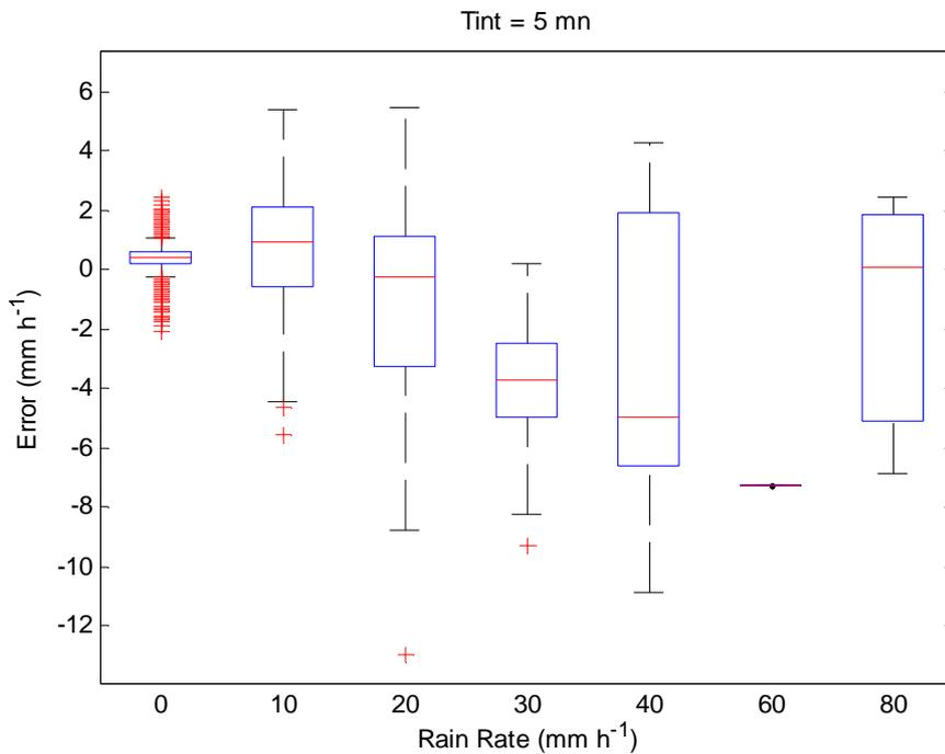
Fig. 2. Error induced on rain estimation when the ITU power law is used for an integration time equal to 5 mn. For each rain bin, the box-and-whiskers diagram indicates the median (the central vertical line), and the lower and upper quartiles (left and right edges of the box). The whiskers indicate the lower and upper limits of the distribution within 1.5 times the interquartile range from the lower and upper quartiles, respectively.
