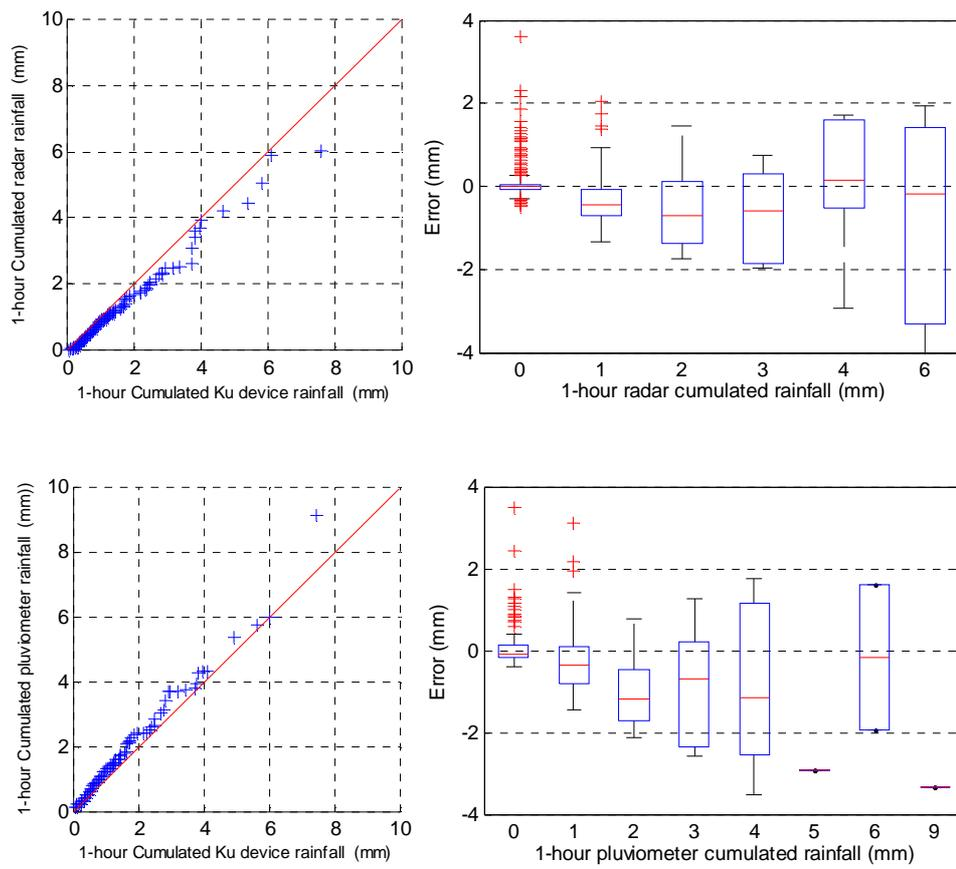
Fig. 11. Q-Q plot between radar and Ku device (top left) and between pluviometers and Ku device (bottom left).
