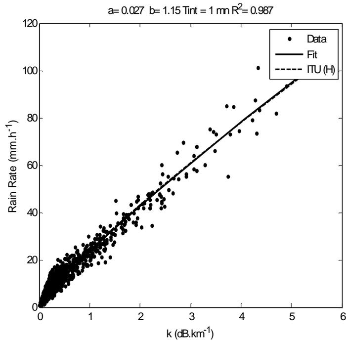
Fig. 1. Scatter plot of rain rate versus specific attenuation computed from drop size distribution and Mie theory for a frequency  $f$  equal to 12 GHz and a time resolution of 1 mn. The continuous line indicates the corresponding fitted  $k$ - $R$  power law. The dotted line indicates the ITU power law for horizontal polarization.
