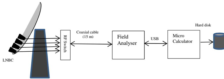
*Fig. 3. Experimental setup.*
