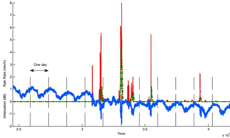
Fig. 5. Example of obtained time series: received signal  $P_{REC}^{chl}(t)$  (blue curve), radar rain rate  $\bar{R}_{chl}^{rad}(t)$  (red curve), 1-hour accumulated rainfall time series  $\bar{R}^{RG}(t)$  (dash green curve)
