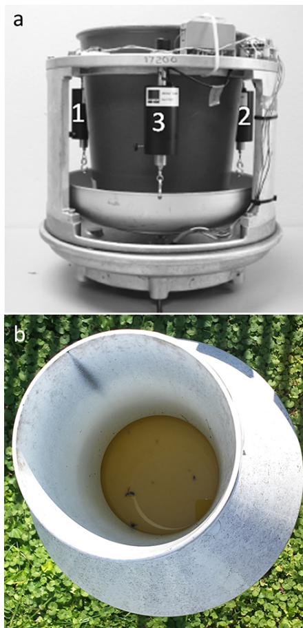
Figure 1. Photographs of the Geonor T200B gauge (a) interior outfitted with redundant sensors and (b) looking through the gauge opening to the exposed interior reservoir.
