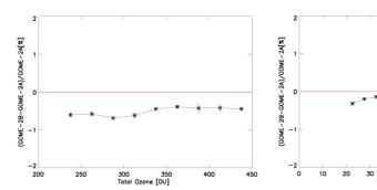
**Fig. 11.** Relative difference between GOME-2A and GOME-2B total ozone columns as a function of total ozone column (left) and solar zenith angle (right). One year (from December 2012 to November 2013) of GOME-2A and GOME-2B data are used.
