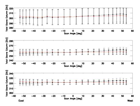
**Fig. 12.** Dependency of GOME-2B total ozone column on instrument scan angle (forward scan only) without (black) and with (red) the empirical scan angle correction for all latitudes (top), tropics (middle) and mid-latitudes (bottom).
