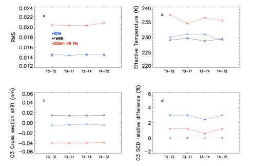
**Fig. 2. (a)** RMS fit residuals, **(b)** Effective temperatures, **(c)**  $O_3$  cross section wavelength shifts **(d)** the change in  $O_3$  slant column relative to the column obtained using GOME FM98 cross sections at 241 K and 221 K (GDP 4.4 settings), obtained after DOAS retrieval of the pixel 5144 of the GOME-2B orbit 5392, using different combination of  $O_3$  absorption cross section data sets. The meanings of T1, T2, T3 and T4 are the same as in Fig. 1.
