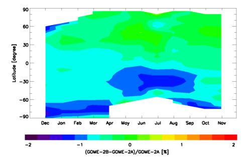
**Fig. 10.** Time series of the zonally mean difference between GOME-2A and GOME-2B total ozone columns from December 2012 to November 2013.
