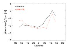
**Fig. 3.** The scan angle dependency of ozone vertical column densities as function of latitude for GOME-2A (2008, black) and GOME-2B (2013, red) for January (left) and June (right). East pixels represent scan angles smaller than 0° and west pixels represent scan angles larger than 0°.
