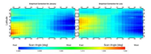
**Fig. 4.** Empirical correction factors as a function of latitude and scan angle (East: scan angle  $< 0^{\circ}$ ; West: scan angle  $> 0^{\circ}$ ) for January and July. Correction ratios larger than one (red) are mostly found for the Eastern part of the scan, while correction factors smaller than one (blue) correspond mostly to the Western part of the scan.
