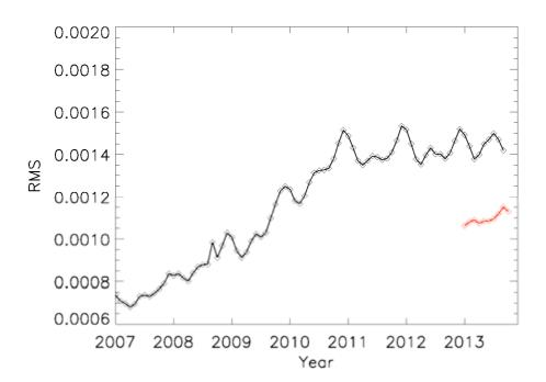
Fig. 7. Long term DOAS fitting residuals for the 325–335 nm ozone fitting window for GOME-2A (black line) and GOME-2B (red line). The monthly averaged residual values have been calculated for the Equator Pacific region (10° S-10° N, 160° E-160° W).
