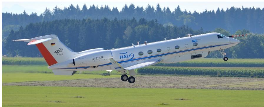
**Fig. 1.** HALO fully equipped during take-off. The image was taken during the preparations for the TACTS campaign. GLORIA is mounted in the belly pod below the aircraft.
