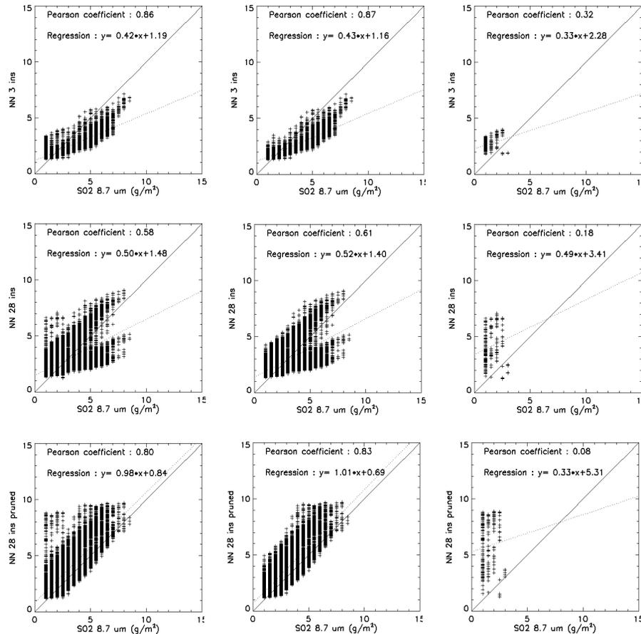
**Fig. 9.** Scatter plots for SO<sub>2</sub> networks, 3 (top row), 28 (middle row) and 28 inputs pruned (bottom row), applied to the validation set of 11 May 2010, 14:05 UTC, divided in total pattern (left column), pattern over sea (middle column), patterns over meteorological cloud (right column).
