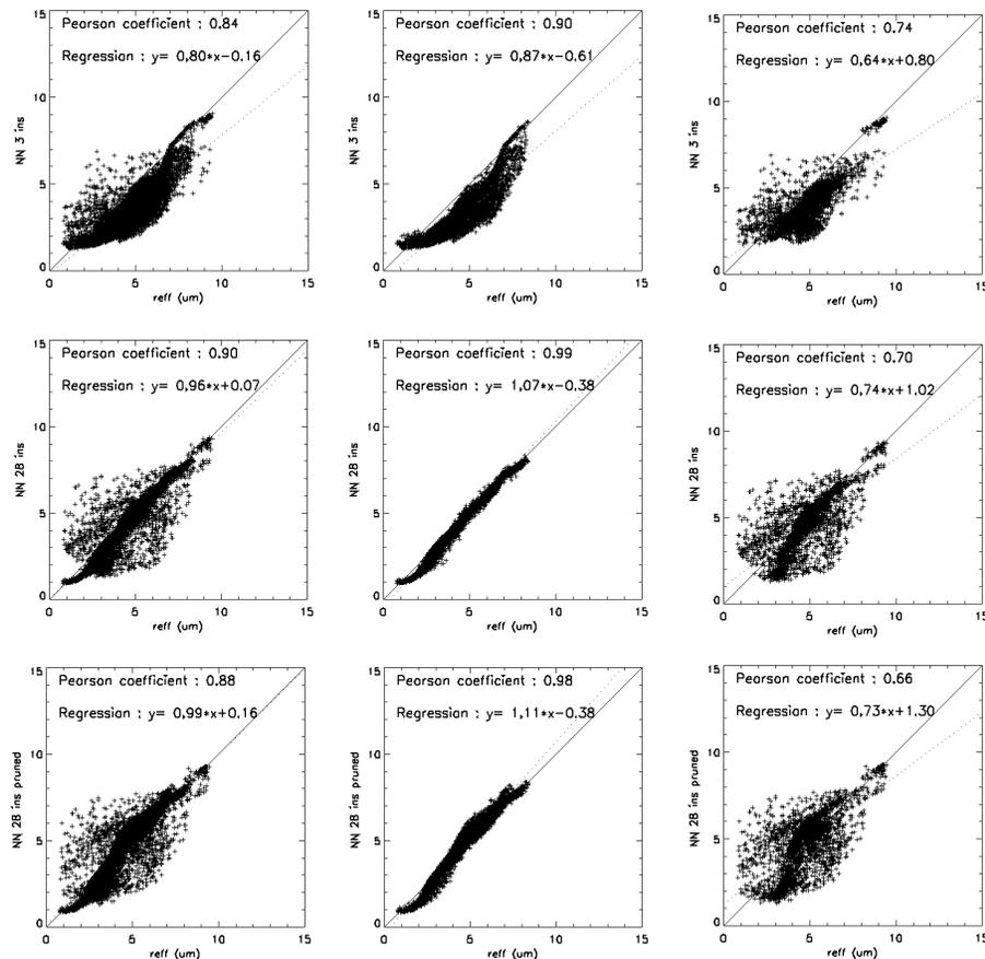
**Fig. 6.** Scatter plots for reff networks, 3 (top row), 28 (middle row) and 28 inputs pruned (bottom row), applied to the validation set of 12 May 2010, 12:55 UTC, divided in total pattern (left column), pattern over sea (middle column), patterns over meteorological cloud (right column).
