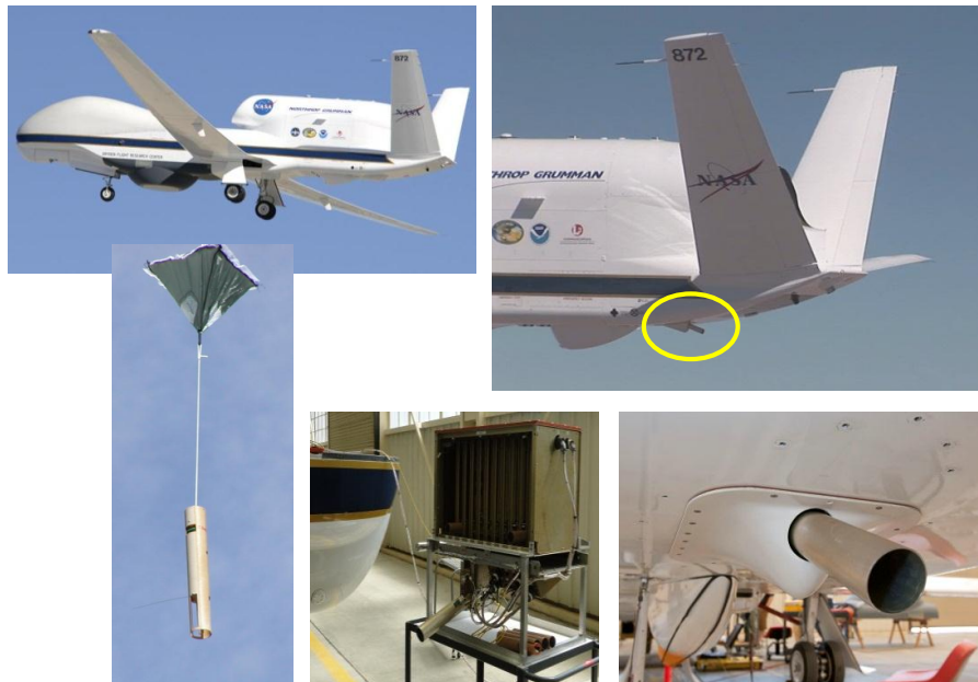
Fig. 1. (Clockwise from top left) Global Hawk; close-up of Global Hawk with dropsonde eject-tub (photo courtesy NASA); close-up of dropsonde launch tube (photo courtesy NASA); dropsonde dispenser and launch assembly; dropsonde with parachute.
