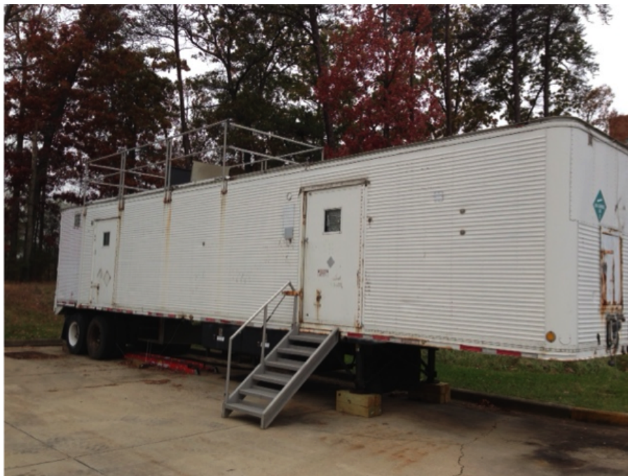
Fig. 4. The 13 m trailer that houses the GSFC TROPOZ DIAL system. The hatch doors are open to transmit the DIAL wavelengths into the atmosphere.
