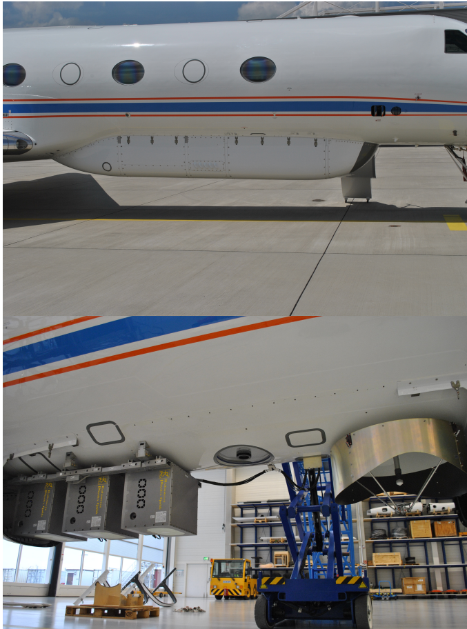
Fig. 1. Top: closed belly pod mounted on HALO. Bottom: remote sensing instruments underneath the body of HALO (from left to right: HALO-G, HALO-KV, and HALO-WF module, lidar window, and cloud radar MIRA-36 antenna).
