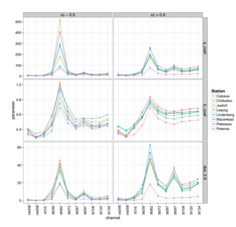
**Figure 6.** Comparison of coefficients *a* (upper panel) and *b* (middle panel) as well as  $dist_{0.9}$  (lower panel) for two different cloud covers (left side half covered scenes and right side fully covered ones) all channels (*x* axes) and locations (different colours).
