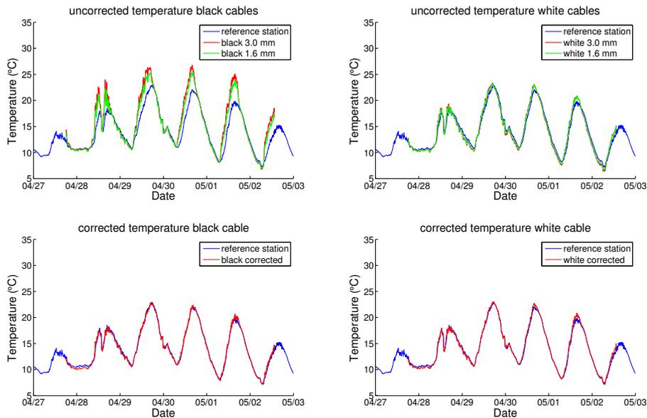
**Figure 2.** Top: comparison between the reference station and the uncorrected averaged temperature of the black (left) and white (right) cables in the measurement section. Bottom: comparison between the reference station and the corrected temperatures of the black (left) and white (right) cable.
