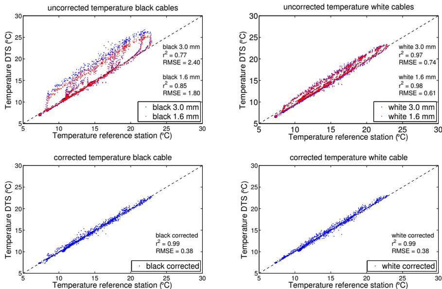
**Figure 3.** Top: correlations between the temperature measurements of the reference station and the uncorrected temperatures of the black (left) and white (right) cable. Bottom: correlation between the temperature measurements of the reference station and the corrected temperatures of the black (left) and white (right) fiber optic cables.
