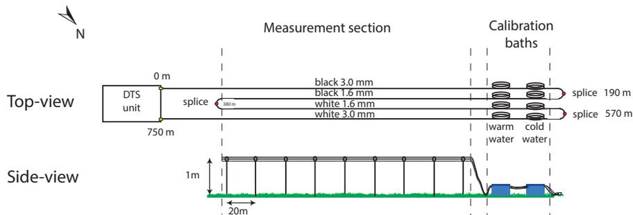
**Figure 1.** Schematic overview of the experimental setup. The cable consisted of four sections (black with diameter 3.0 mm and 1.6 mm and white with diameter 3.0 mm and 1.6 mm). In the measurement section the cables are held in open air above a grass field.
