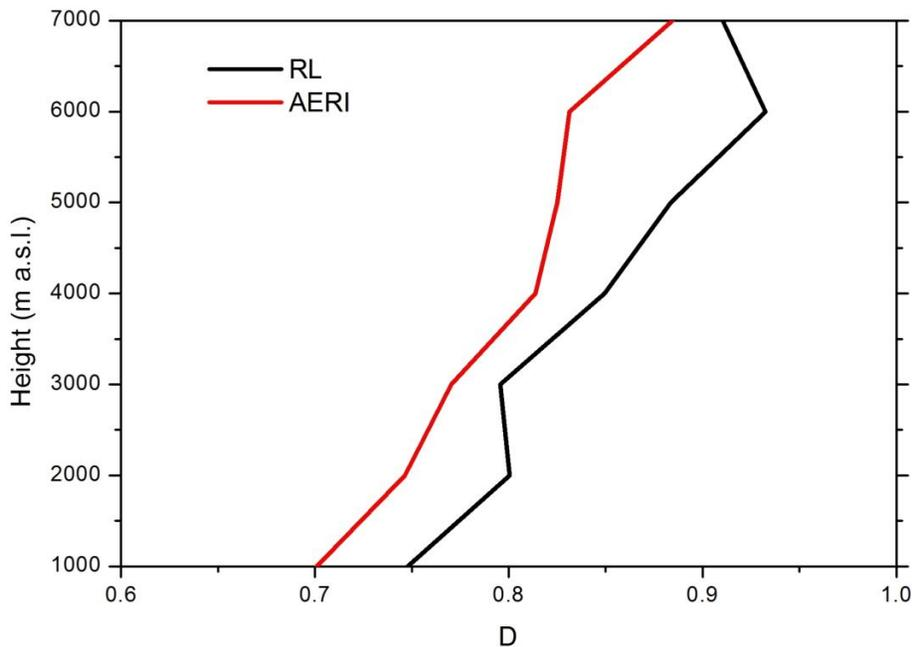
**Figure 5.** Comparison of the statistical distances retrieved for the three instruments (Raman lidar [RL], Atmospheric Emitted Radiance Interferometer [AERI], and RS92 radiosonde) measuring the water vapor vertical profile at the Southern Great Plains (SGP) site. The data set considered includes all measurements available at SGP (144 profiles) in the period 2010–2012.
