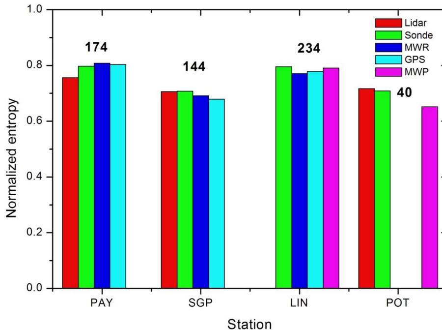
**Figure 3.** Comparison of the normalized entropy retrieved for the instruments measuring integrated water vapor at the Lindenberg (LIN), Payerne (PAY), Potenza (POT), and Southern Great Plains (SGP) sites. The data set considered includes all available measurements in 2010–2012. The numbers above the bars represent the number of cases selected, according to the quality assurance criteria for each station.
