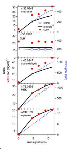
Figure 5. Signal, (signal)<sup>1/2</sup>, and standard deviation of the signal (noise) during a typical PTR-TOF calibration measurement for some selected masses.
