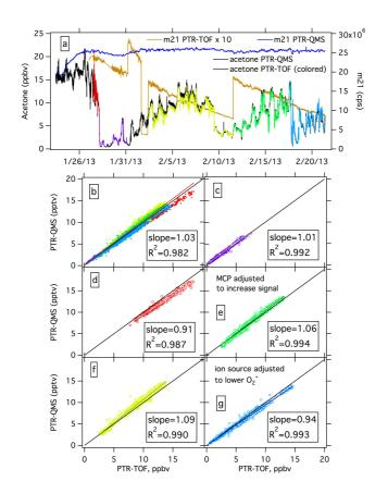
Figure 7. PTR-QMS and PTR-TOF acetone inter-comparison during UBWOS2013: (a) time series of the PTR-TOF and PTR-QMS primary ions and acetone. The color code of the PTR-TOF acetone signal indicates, when the PTR-TOF was relatively stable. (b) Scatter plot of PTR-QMS and PTR-TOF acetone for the whole campaign. (c-q) Scatter plots for separate stable periods of the PTR-TOF.
