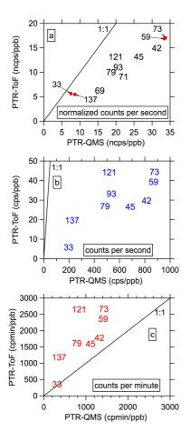
**Figure 3.** (a) PTR-QMS and PTR-TOF sensitivity in ncps ppbv $^{-1}$  normalized to 1 × 10 $^6$  H $_3$ O $^+$  ions. (b) Sensitivity in cps ppbv $^{-1}$  with PTR-QMS 25 × 10 $^6$  and PTR-TOF 1.6 × 10 $^6$  H $_3$ O $^+$  ions. (c) Sensitivity in cpmin ppbv $^{-1}$  with PTR-QMS measuring 37 ions. The numbers in (a), (b) and (c) are the nominal mass of the calibrated compounds.
