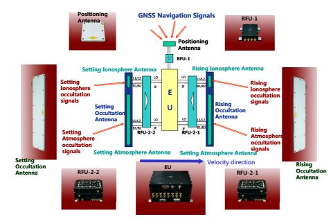
Fig. 1. GNOS instrument configuration.
