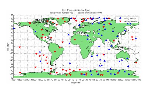
**Fig. 2.** Global distribution of GNOS Beidou occultation events in 24 h simulation. Upward-pointing triangle triangles denote rising occultations. Downward-pointing triangles denote setting occultations.
