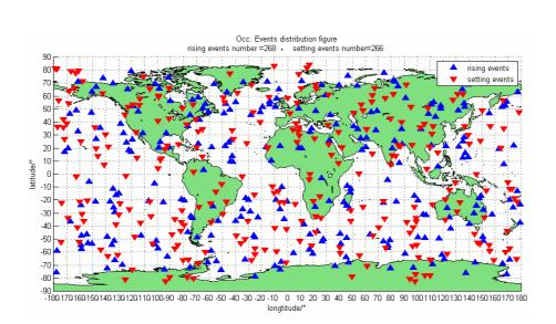
**Fig. 3.** Global distribution of GNOS GPS occultation events in 24 h simulation. Upward-pointing triangle triangles denote rising occultations. Downward-pointing triangles denote setting occultations.
