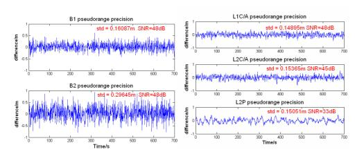
**Fig. 4.** The example of GNOS pseudorange measurement precision for Beidou and GPS. The left panel shows the B1 and B2 peseudorange measurement precision. The right panel shows the L1C/A, L2C/A and L2P peseudorange measurement precision, respectively.
