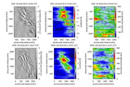
**Figure 8.** Spectral analyses for two satellite overpasses of IASI (top) and AIRS (bottom) during the mountain wave event shown in Fig. 7. Data are shown on the along-track and across-track measurement grid, with a descending orbit for IASI and an ascending orbit for AIRS. Black contour lines indicate areas with wave amplitudes larger than 1 K.
