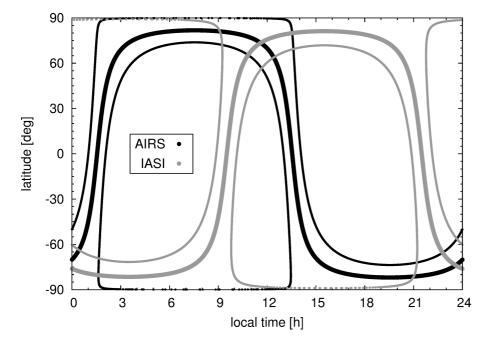
**Figure 1.** Local time vs. latitude of AIRS and IASI observations. Thick curves represent the nadir measurement track. Thin curves represent the outermost measurement tracks. AIRS and IASI have sun-synchronous orbits, which combine orbit altitude and inclination in such a way that the satellite ascends or descends over any given latitude at the same local time. The orbit parameters stay constant over the time period of the mission.
