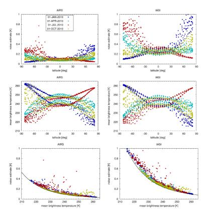
**Figure 6.** Noise estimates (top) and mean scene temperatures (middle) as a function of latitude as well as correlation plots of noise and scene temperatures (bottom) for AIRS (left) and IASI (right). Individual dots represent mean values for boxes of about 2000 km  $\times$  2000 km. Colors refer to different days of measurement. Black curves show scaling of NEDT with scene temperature.
