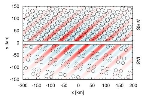
Figure 2. Illustration of the scan patterns of AIRS (upper half of plot) and IASI (lower half) close to the nadir direction. Contour surface in the background shows a wave pattern with 50 km horizontal wavelength. Circles show individual footprints (diameter represents their size). We refer to the distance between the footprints as "spatial sampling" and we refer to the size of the footprints as "spatial resolution".
