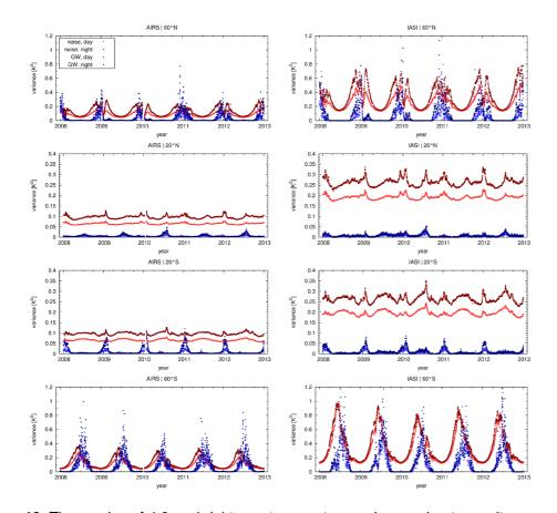
Figure 12. Time series of 4.3 µm brightness temperature variances due to gravity waves and noise estimates for AIRS (left) and IASI (right) at different latitudes (see plot titles). Note that the range of variances shown here differs between the lower and higher latitudes.
