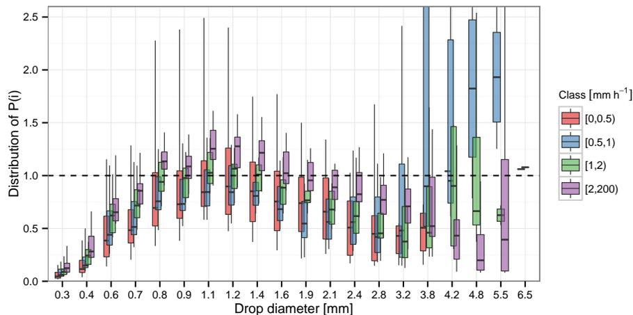
**Figure 8.** Distributions of  $P(i)$  values classed by Parsivel-derived intensity. The correction factors used are the medians of the distributions. The boxes show the interquartile-ranges while lines show the 10% to 90% quantiles of each distribution. The y axis is cut at 2.6.
