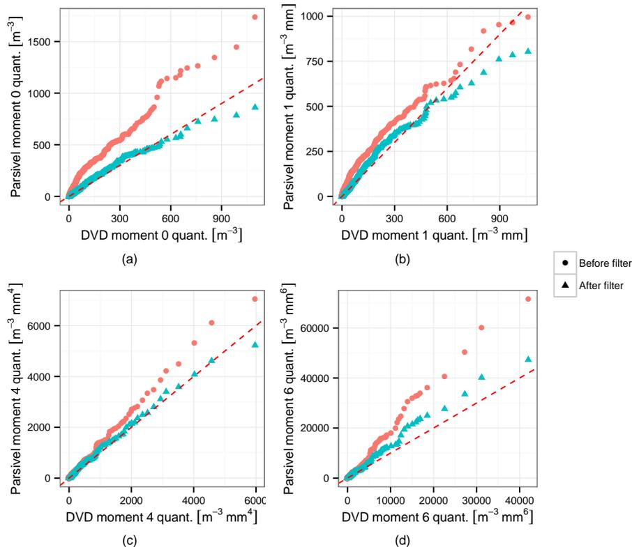
**Figure 12.** QQplot showing the effect of the correction on Parsivel DSD moments (a) zero, (b) one, (c) four, and (d) six, by comparing to the 2DVD moments, for HYMEX SOP 2013 event time steps at Pradel Grainage.
