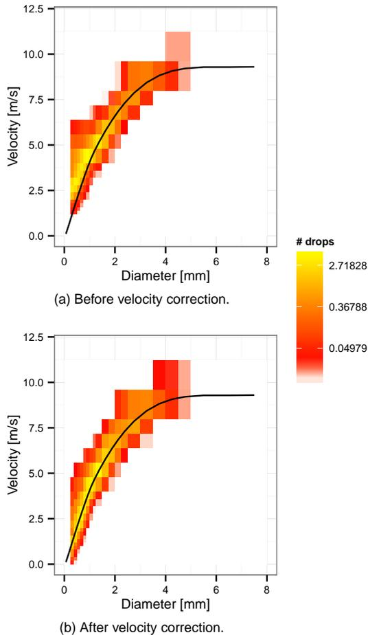
**Figure 6.** An example of the velocity correction. Average drop counts for the Parsivel at Pradel Grainage for SOP 2013, shown **(a)** before the velocity correction and **(b)** afterwards.
