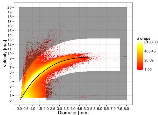
**Figure 3.** Occurrence of velocity/diameter combinations, with drop counts on a log scale, recorded by 2DVD during the HYMEX campaigns in the autumns of 2012 and 2013. The physical-drop filter is overlaid in grey. The black line indicates the Beard 1976 expected terminal drop velocity.
