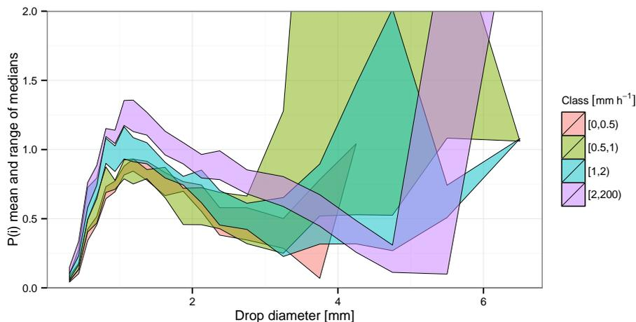
**Figure 9.** Sampling effect per diameter class, for different classes of Parsivel-derived intensity. The coloured regions represent the minimum and maximum median  $P(i)$  per equivolume drop diameter class observed over 100 iterations. The y axis is cut at 2.6.
