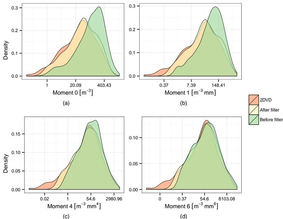
**Figure 11.** The effect of the correction DSD moments (a) zero and (b) one, (c) four, and (d) six, showing the densities of the Parsivel-derived DSD moments before and after the correction was applied, and the 2DVD moments, for HYMEX SOP 2013 event time steps at Pradel Grainage. The x axis has a log scale.
