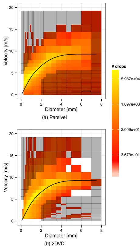
**Figure 4.** Sum of raw drop occurrences per Parsivel class, for the 2012 and 2013 campaigns. Parsivel counts are summed at stations Pradel 1 (for 2012) and Pradel Grainage (for 2013). The filtered areas are overlaid in grey. The black line is the expected terminal drop velocity calculated by Beard (1976). Drop counts are specified by colour on a log scale.
