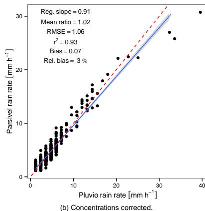
**Figure 13.** Scatterplots showing the effect of the drop concentration correction, for the combined SOPs, with liquid precipitation only and rain rates over  $1.2 \text{ mm h}^{-1}$ , for Pradel 1, the closest station to the 2DVD that was present in both 2012 and 2013.
