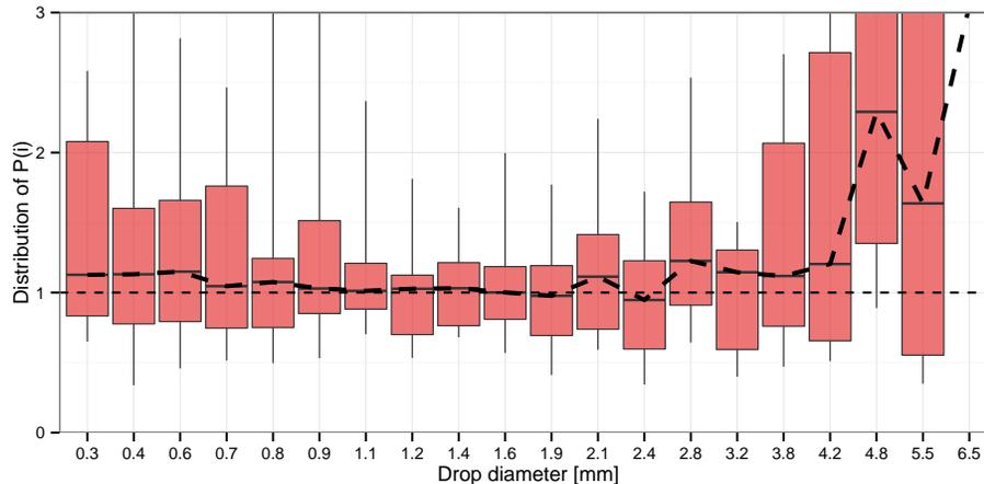
**Figure 10.** The distributions of  $P(i)$  values for the corrected DSD, on an example set of validation time steps from HyMeX 2013, and for all classes of Parsivel-derived intensity, for the Parsivel collocated with the 2DVD. The y axis is cut at 3.
