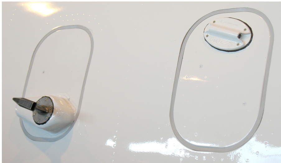
Figure 1. External view of WVSS-II fitted to FAAM aircraft showing the two inlets (Rosemount, left, flush right) angled down to match the local air flow in flight.
