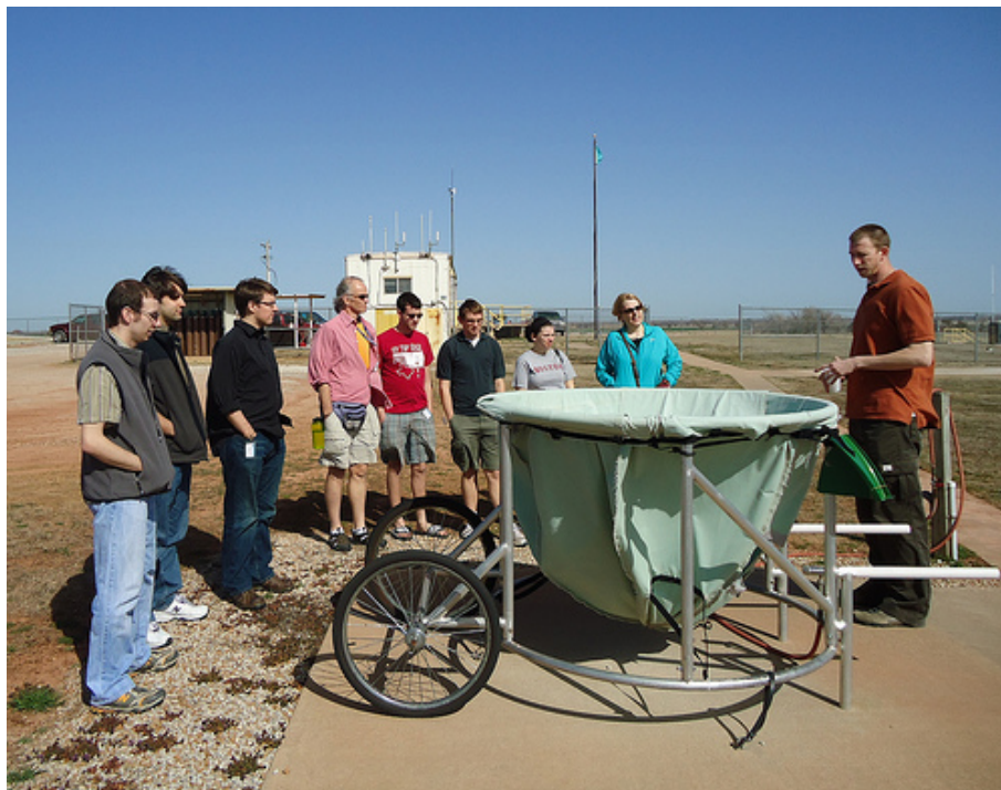
Figure 2. SGP sounding launch ARM SGP staff explains the launch process for the balloon borne sounding system (or weather balloons) using the custom made “launch cart” at the ARM Southern Great Plains site.
