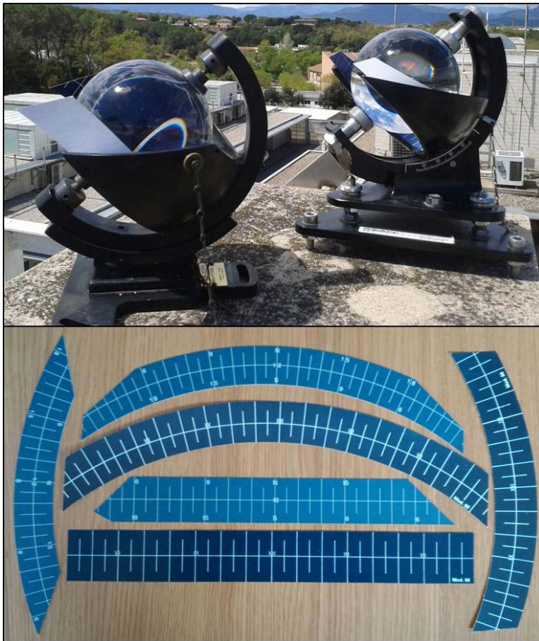
Figure 2. (a) Details of the two different CSSRs mounted in Girona (NE Spain), and (b) an example of the 3 types of cards used during summer, winter and equinoctial seasons, respectively (the longer the daylight hours, the longer the card).
