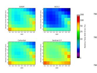
**Fig. 9:** Relative AOD error as a function of aerosol centre height and AOD for the parameterised aerosol retrieval for a SZA of  $30^{\circ}$  and albedo of 0.5. Intensity offset is included.
