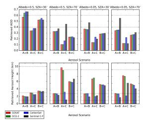
**Fig. 10:** AOD and height errors for the parameterised aerosol retrievals for the combined aerosol scenarios A+B, A+C and B+C. In the top row the horizontal lines indicate the true AOD values for each case, i.e. the sum of both layers. In the bottom row they show the heights of each individual layer as a reference noting that the prior value for each scenario is the lowest layer height.
