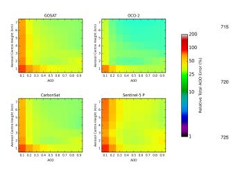
**Fig. 8:** Total AOD error (given as a relative error) as a function of aerosol centre height and AOD for the four instruments for a SZA <sup>730</sup> of  $30^{\circ}$  and albedo of 0.5. Intensity offset is included in the retrieval.
