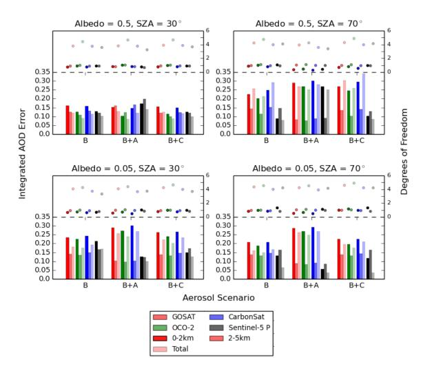
**Fig. 6:** AOD error and DoF for the aerosol profile retrieval for surface albedos of 0.05 and 0.5 and SZAs of 30° and 70° for the four instruments. Errors are integrated over the 0-2 km and 2-5 km ranges as well as the total column for aerosol scenario A and combined aerosol scenarios A+B and A+C. Intensity offset is included.
