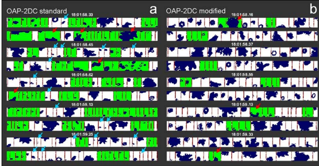
Figure 56. Examples of the results of the image rejection/acceptance processing with the inter-arrival time algorithm. The images of ice particles were simultaneously sampled by the standard (left) and modified (right) OAP-2DC during the time period shown in Fig.45. Green backgrounds highlights the images identified by the inter-arrival time algorithm as artifacts. Images with a white background were accepted by the algorithm. As seen in (a) in some cases the standard OAP-2DC rejects large particles which appear to be intact (red arrows), at the same time it accepts particles, which have the features of shattered fragments (blue arrows).
