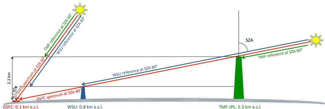
**Fig. 2.** DS DOAS “analysis geometry” to detect O<sub>2</sub>O<sub>2</sub> absorption within PBL (2.2 km and 680 m) only.
