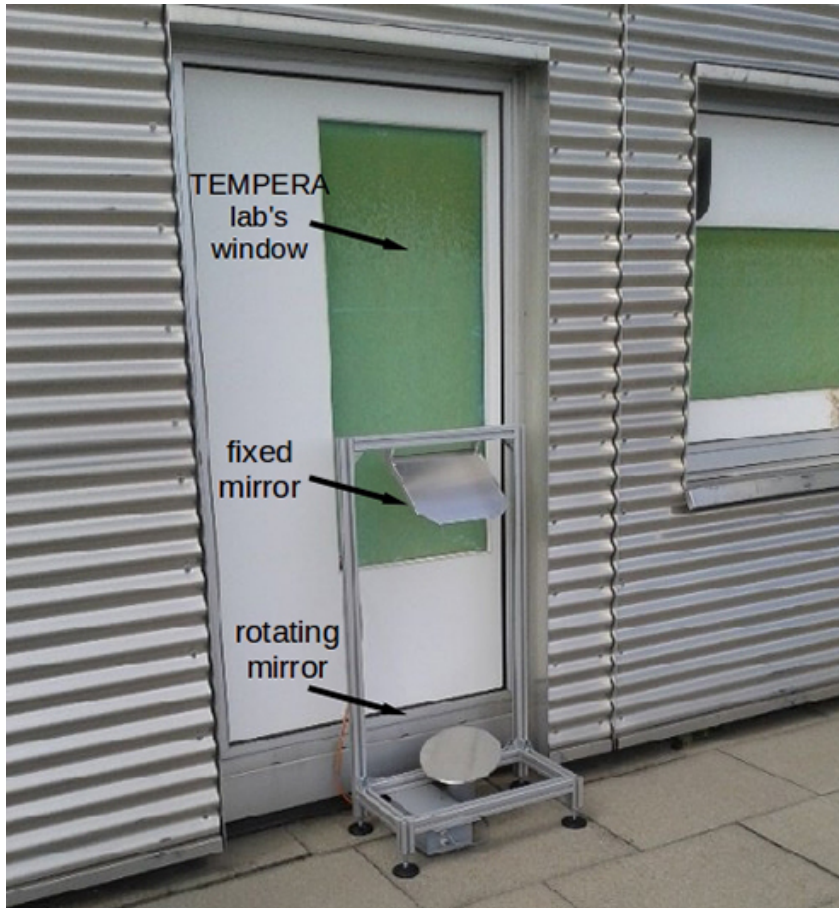
Figure 3. Secondary mirror installed on the roof of the ExWi Building at the University of Bern.
