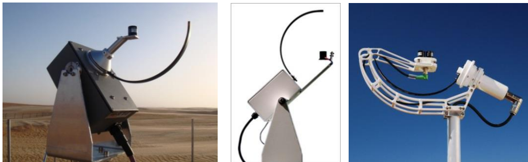
Figure 1. Rotating Shadowband Irradiometers. Left: RSR2 (irradiance Inc.), center: RSP4G (Reichert GmbH), right: Twin-RSI (CSP Services GmbH) (Wilbert et al., 2015).
