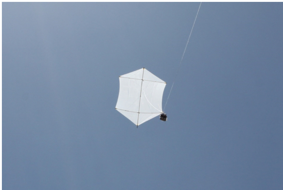
Figure 2. View of the kite and lightweight PTU probe used for lidar calibration.
