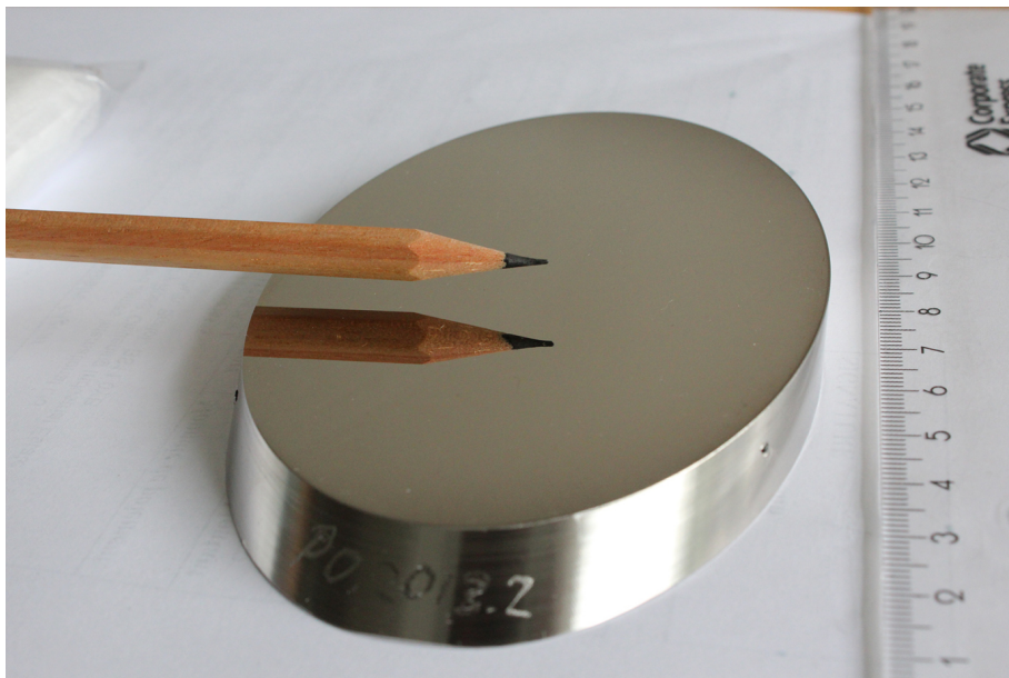
Figure 7. Stainless steel mirror with lapped and polished optical grade surface.
