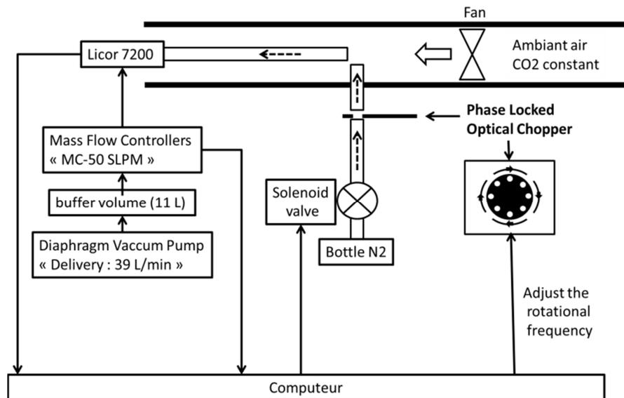
**Figure 1.** Calibration bench for cut off frequency determination.
