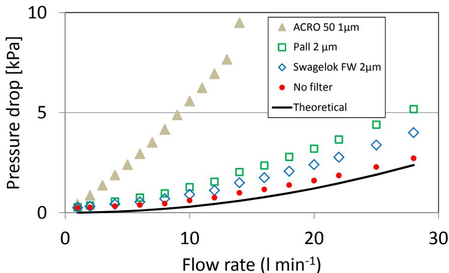
**Figure 3.** Pressure drop in the IRGA cell (kPa) in function of the flow rate ( $\text{Lmin}^{-1}$ ) for different filters ACRO-50 (triangles), Pall  $2\ \mu\text{m}$  (crosses), Swagelok FW  $2\ \mu\text{m}$  (diamonds), and without any filter (asterisks). The theoretical curve (Eq. 1) is given by the continuous line.
