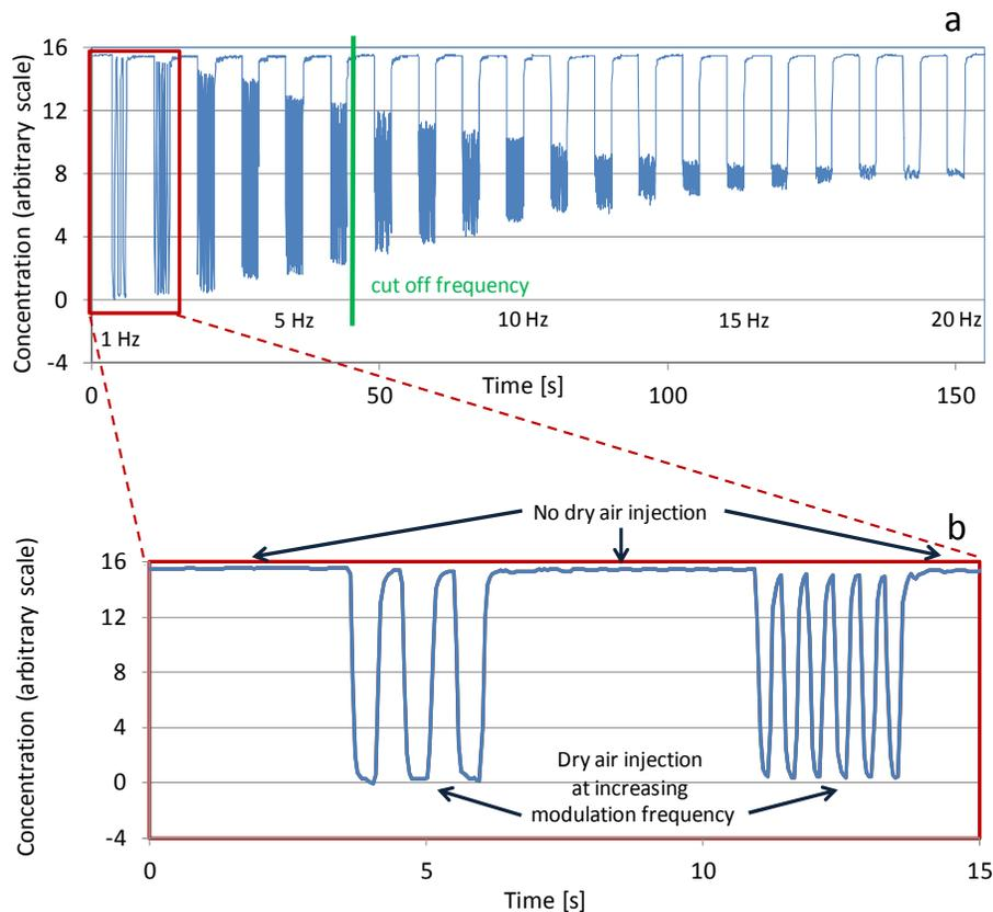
**Figure 2.** Recording of concentration measurements by the IRGA during one measurement cycle. **(a)** Representation of the whole cycle. **(b)** Focus on the first 15 s. For details, see text.
