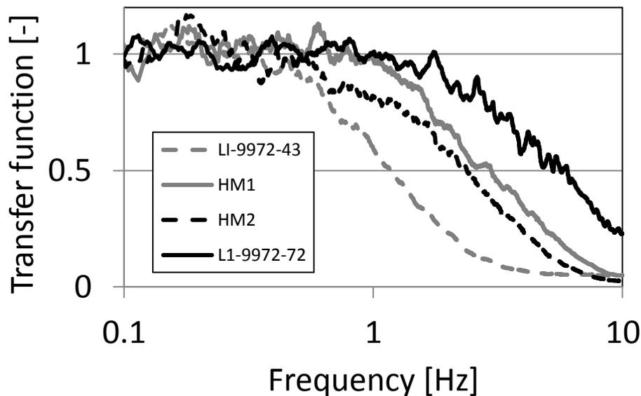
**Figure 5.** Transfer functions corresponding to different rain cup designs. Legend: dotted grey line: LI-9972-43; dotted black line: HM1; full grey line: HM2; full black line: LI-9972-72.
