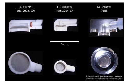
**Figure 1.** Three selected rain cap designs tested in this study. Top row: cross-sections of each rain cap showing their internal volumes. Bottom row: rain cap inlets with screens that face downwards in typical field deployments.
