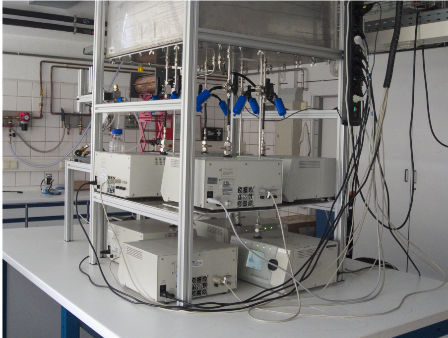
Figure 1. Photo of the measuring setup for the intercomparison of eight units APS 3321.
