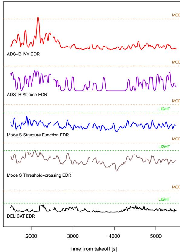
**Figure 7.** Results for FL8 for all analysed approaches to estimate EDR and a reference EDR (as in Fig. 2). The time series are scaled to match the intensity of the FL9 MOD event. For reference the tentative turbulence levels have been added to the plot. Those are reflecting the FL9 encounters and levels of noise inferred from the calm flights.
