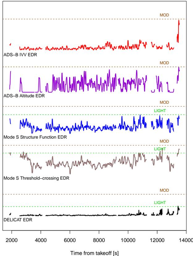
**Figure 8.** Results for FL6 for all analysed approaches to estimate EDR and a reference EDR (as in Fig. 2). The time series are scaled to match the intensity of the FL9 MOD event. For reference the tentative turbulence levels have been added to the plot. Those are reflecting the FL9 encounters and levels of noise inferred from the calm flights.
