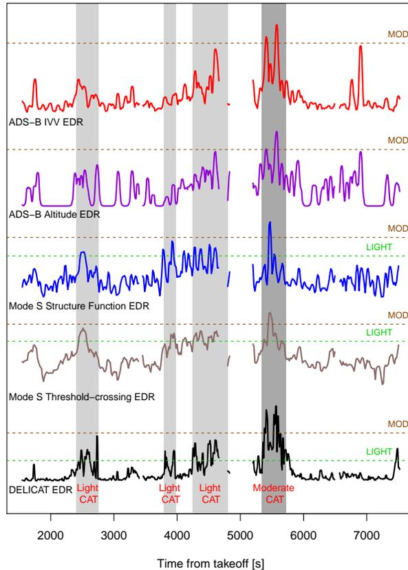
**Figure 6.** Results for FL9 for all analysed approaches to estimate EDR and a reference EDR (as in Fig. 2). The time series are scaled to match the intensity of the MOD event. For reference the tentative turbulence levels have been added to the plot. Those are reflecting the FL9 encounters and levels of noise inferred from the calm flights.
