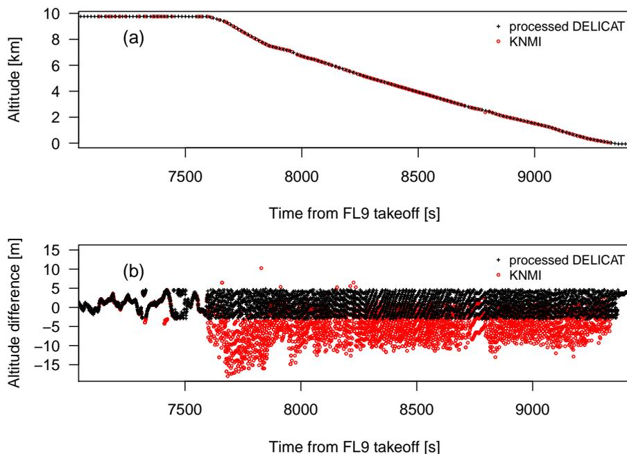
**Figure 3.** A comparison between the processed DELICAT data (black crosses) and KNMI data (red circles) of **(a)** the altitude profile (note that for the sake of clearness 97 % of the observations are not plotted here) and **(b)** the difference of the altitude with respect to the DELICAT reference altitude.
