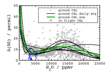
**Figure 4.** Uncertainty analysis for all flight days. Grey symbols: deviation of individual 1 Hz calibration measurements from calibration standard; black lines: daily fit of  $\Delta(\delta D)$  (Eq. 2); green line: campaign average of  $\Delta(\delta D)$ . In-flight calibrations are depicted as the difference to the daily mean (absolute value) by the blue symbols.
