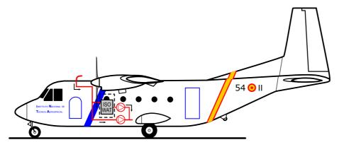
**Figure 7.** CASA C-212 aircraft of Instituto Nacional de Técnica Aerospacial (INTA). The rearward-facing ambient air inlet was located on top of the fuselage. The inlet line was flushed at a high flow using a membrane pump. ISOWAT was mounted in the foremost position of the aircraft and was equipped with a second pump to establish the gas flow through the instrument.
