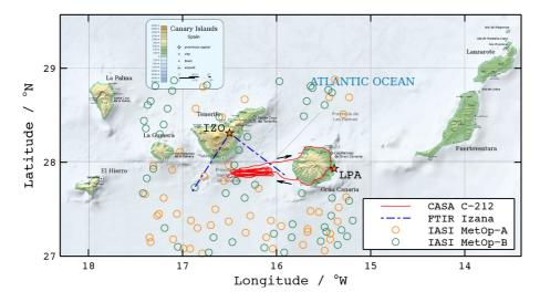
**Figure 6.** Aircraft flight track (red) of 24 July 2013 departing from Las Palmas Airport (LPA). Also shown are all Metop A and Metop B measurements (symbols) obtained during the campaign after a data-quality filter was applied. The FTIR line of sight (blue lines) for 10:30 and 13:00 UTC (start and end of profile measurements) at Izaña (IZO) is indicated. (Map source: http://en. wikipedia.org/wiki/File:Map\_of\_the\_Canary\_Islands.svg)
