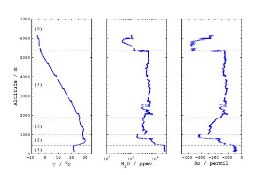
**Figure 10.** Measurements of temperature (*T*),  $H_2O$  mixing ratio, and  $\delta D$  taken with 1 s averaging on 31 July 2013. The profile is divided into 5 layers for interpretation.
