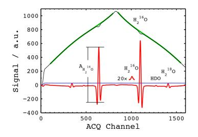
**Figure 2.** Example spectra of ISOWAT II showing the up and down scan across the absorption region of interest. Polynomial baseline (green trace) of the direct absorption spectra (black trace) as well as detector zero signal (blue trace) are used to normalize the second-harmonic absorption spectra (red trace).  $A_{H_2}{}^{16}O$  is the peak-to-peak amplitude of the strong  $H_2{}^{16}O$  absorption line. The weak  $H_2{}^{16}O$  line used in humid conditions is depicted 20× enlarged.
