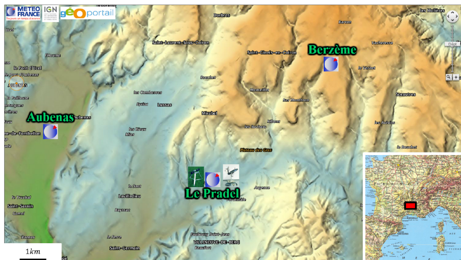
Figure 2. Location of the studied area in the south-east of France, on a topographic map. The two instruments used in the assimilation algorithm (MRR and DBS, see Sect. 3.1 and 3.2) are located at Le Pradel, 278m height. The 3 automatic Météo France weather stations of Le Pradel (same place), Aubenas (7.5km westward, 180m height) and Berzème (7.5km on the north-east, 650m height) are also shown.
