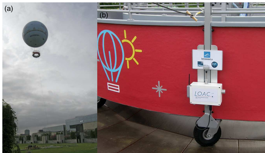
Figure 7. LOAC on the recreational OAG tethered balloon in Parc André Citroën, Paris. From left to right: (a) view on the balloon in flight; (b) view of the LOAC installed in a small box on the side of the passenger gondola with its TSP inlet above, a small WiFi antenna on the left of the box for data transmission, and a ventilation opening protection (grey) on the right.
