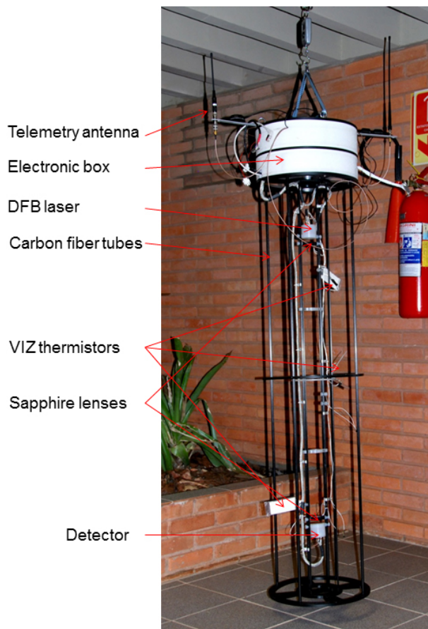
Figure 1. Description of the Pico-SDLA H 2 O hygrometer, improved for the TRO-Pico campaign (2012–2013).
