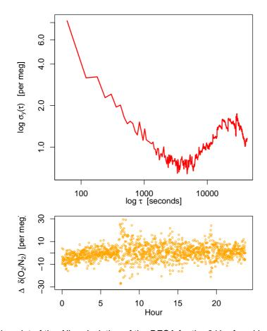
Figure 3. Log-log plot of the Allan deviation of the DFCA for the 24 h of working tank flow (top panel) and anomaly of  $\delta(O_2/N_2)$ , calculated as the instantaneous data minus the mean of the whole test (bottom panel).
