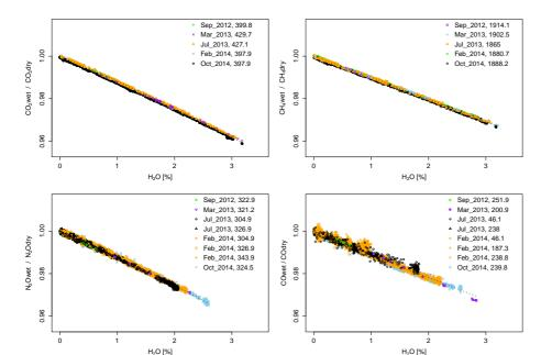
**Figure 4.** Water correction functions from different tests for all measurands. Colors represent different dates, and shapes represent specific mole fractions of the cylinder used for the test, all in ppb, except for CO<sub>2</sub>, which is in ppm.
