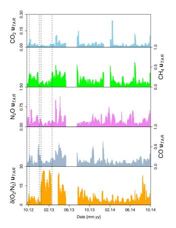
**Figure 6.** Measurement uncertainty derived from target measurements ( $u_{tar}$ ). Mean bias (i.e., differences from MPI-BGC determinations of target tank concentration from NDAO's determination) for each tank has been removed to better approximate the sample uncertainty. Dashed vertical lines indicate a target tank change.
