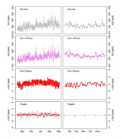
**Figure 7.** Detail of the working tank correction for the OA-ICOS instrument, showing the correction process for the entire time series (left) and an arbitrarily selected week (right). Gray points are uncorrected data, and red are corrected data.
