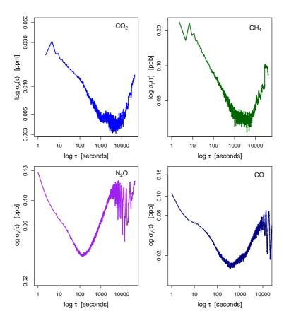
**Figure 2.** Log-log plots of the Allan deviations of the output of the CRDS and OA-ICOS instruments as they received gas flow from a working tank for 24 h.
