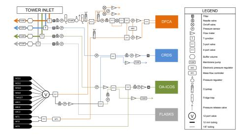
**Figure 1.** Diagram of the measurement system.
