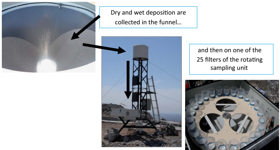
Figure 2. CARAGA sampling system of total insoluble atmospheric deposition installed on Frioul Island (43.27° N; 5.29° E).
