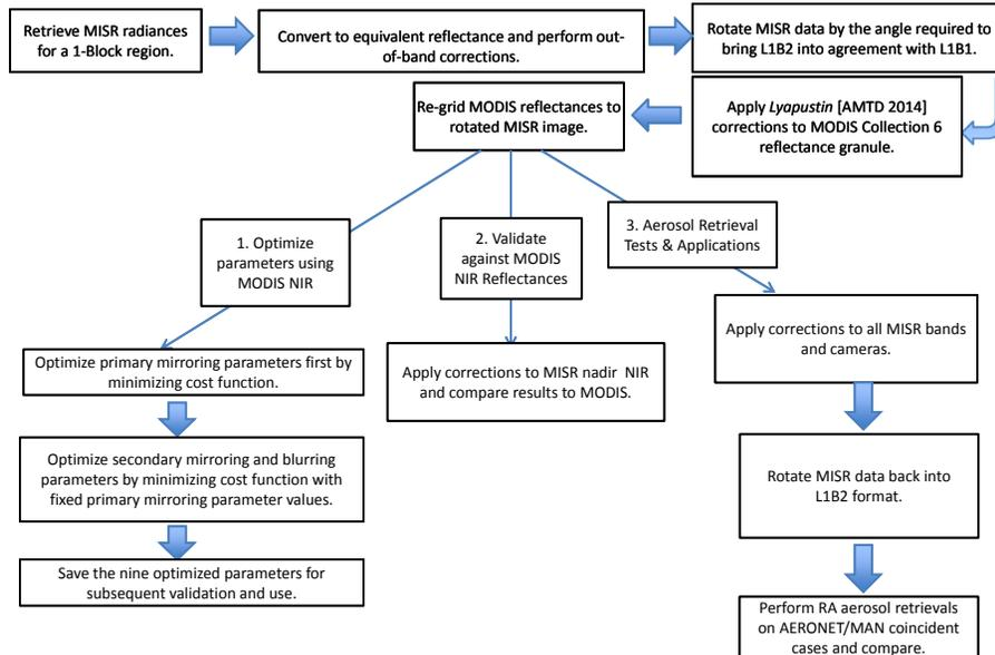
**Figure 5.** Flow-chart summarizing the steps involved in the MISR internal reflection correction.
