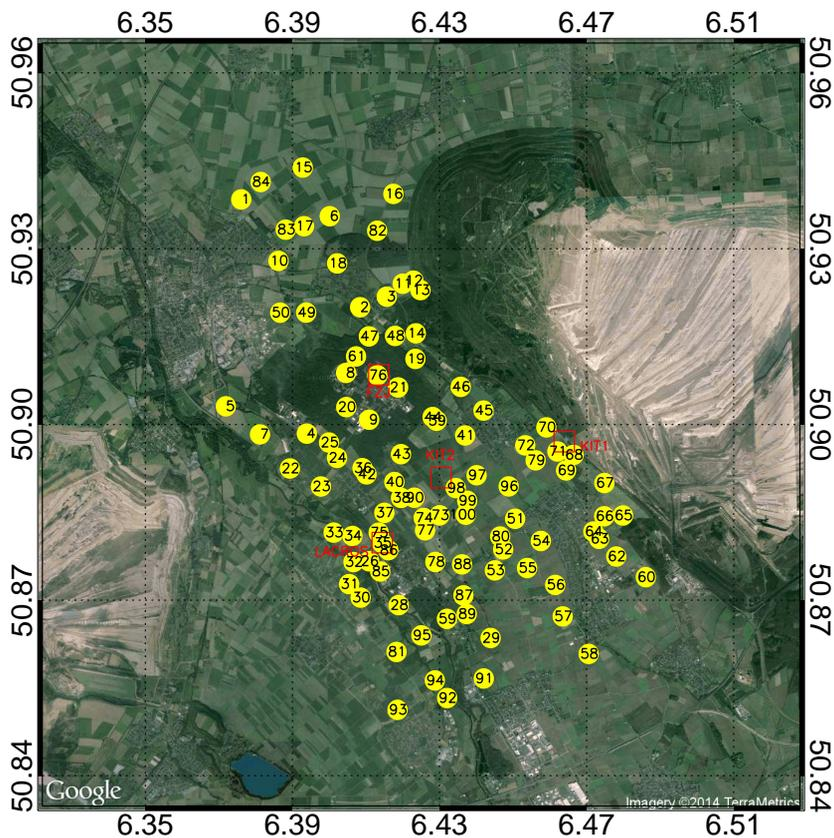
**Figure 2.** Spatial distribution of pyranometer network during HOPE campaign. Each yellow circle represents a pyranometer station with a unique station identification number. Collocated sites with additional measurements from thermopile pyranometers and a sky imager are marked in open red squares. (Source for background image: Google.)
