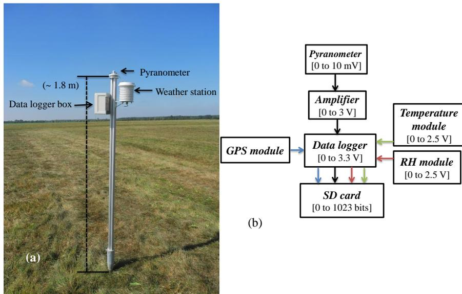
**Figure 1.** (a) Picture of a pyranometer station in the field, and (b) the flow diagram for data recording.
