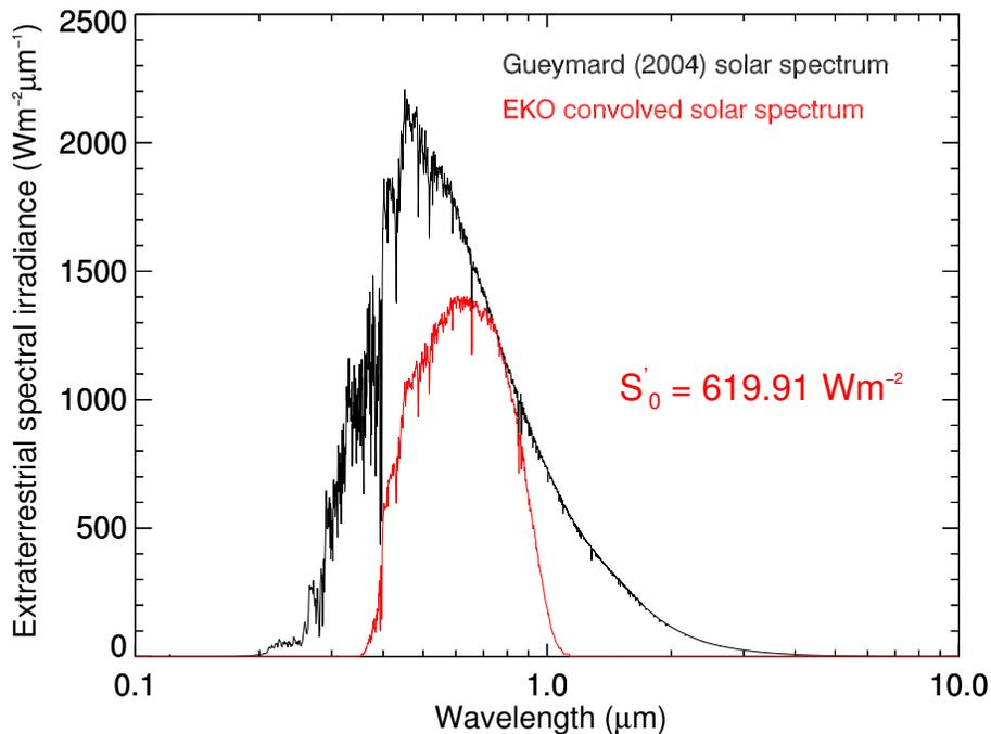
**Figure 3.** Extraterrestrial solar spectrum of Gueymard (2004) weighted by the spectral response function of the EKO ML-020VM silicon photodiode sensor.
