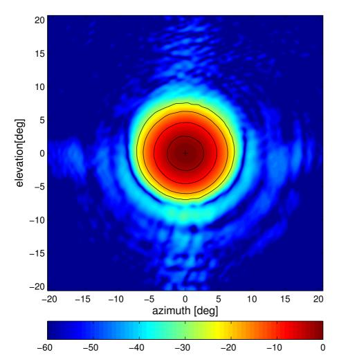
**Figure 5.** Farfield antenna pattern for the GROMOS-C beam pointed at horizon. 3034
