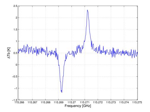
**Figure 19.** CO balanced spectrum measured with GROMOS-C by fast frequency switching and calibrated with hot and Peltier loads. The elevation angle is 30° and the integration time was 8 h.
