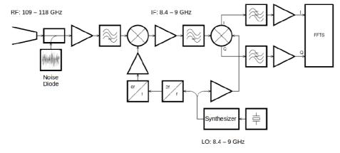
Figure 8. Block diagram of GROMOS-C receiver.
