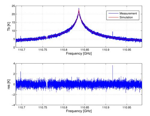
**Figure 16.** Above, measured and simulated one day ozone spectrum; below, residuals between simulation and measurement.
