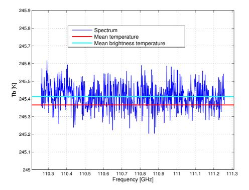
**Figure 11.** Peltier load brightness temperature integrated during four hours, calibrated with liquid nitrogen and a hot load. The red line represents the average temperature measured by the sensors on the wedge, and the cyan line is the average brightness temperature.
