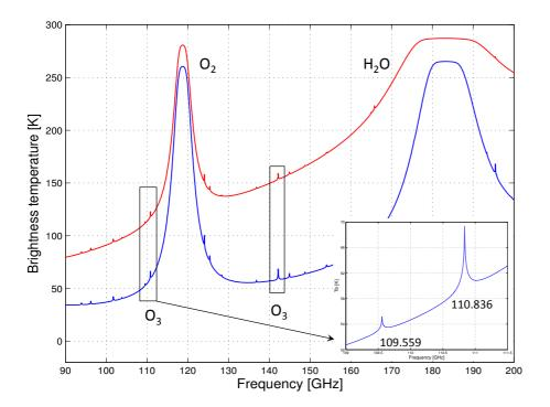
**Figure 1.** The emission spectrum of a midlatitude standard atmosphere in winter (blue) and summer (red), for an elevation angle of 45° and an altitude of 500 m, simulated with ARTS. The ozone lines are highlighted.
