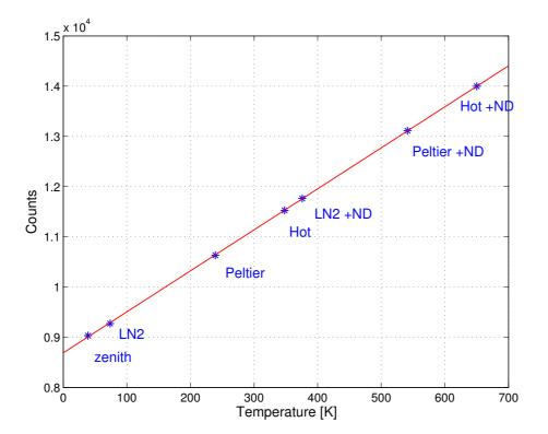
**Figure 9.** All the different calibration loads plotted vs. the counts measured by the spectrometer. The linear regression by least-square fit gives an  $R^2 = 0.9999$ .
