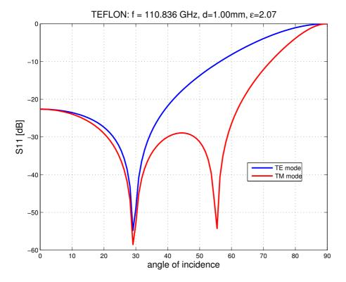
**Figure 4.** Reflection parameter for 1 mm thick teflon, simulated with Fresnel equations at the nominal frequency and for different incidence angles. The red line corresponds to the case of transverse-magnetic (TM) polarization and the blue to transverse-electric polarization (TE). We observe in both cases a strong resonance at 29°. For the TM mode the second resonance corresponds to the Brewster angle.
