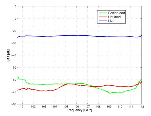
**Figure 12.** S<sub>11</sub> measured for the Peltier, hot and liquid nitrogen targets with the vector network analyzer for the frequency interval 100–112 GHz.
