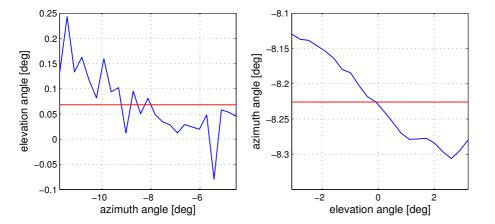
Figure 7. Pointing offsets obtained from the Sun scanning of GROMOS-C at Junfraujoch.
