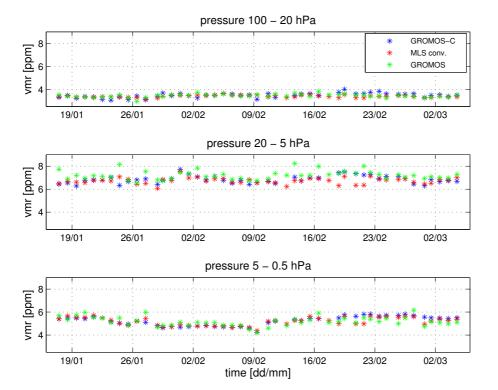
**Figure 18.** Timeseries of ozone volume mixing ratio for 3 pressure levels, retrieved by GROMOS-C and compared with MLS convolved, during the Jungfraujoch campaign.
