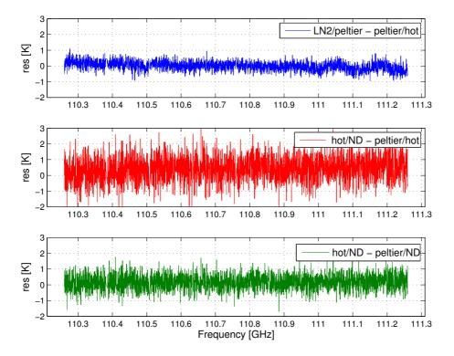
**Figure 15.** Residuals, corresponding to differences between the spectra calibrated with different loads in Fig. 14. The first always indicates the corresponding load used as cold load whereas the second indicates the hot load. Note the hot load can be used as a cold load and viceversa.
