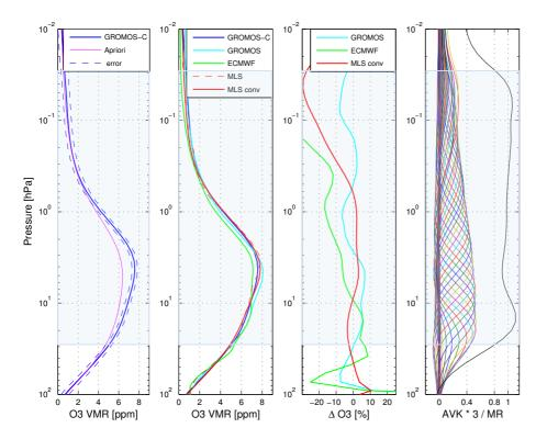
**Figure 17.** Example of an ozone vertical profile retrieved from a daily mean spectrum (21 January 2014), plotted together with the a priori profile and the total error limits. A comparison of the profile with MLS, GROMOS and ECMWF is shown in the middle plots. The averaging kernels and the measurement response are shown on the right side plot. The shadow covers the altitudes where the measurement response is bigger than 0.8.
