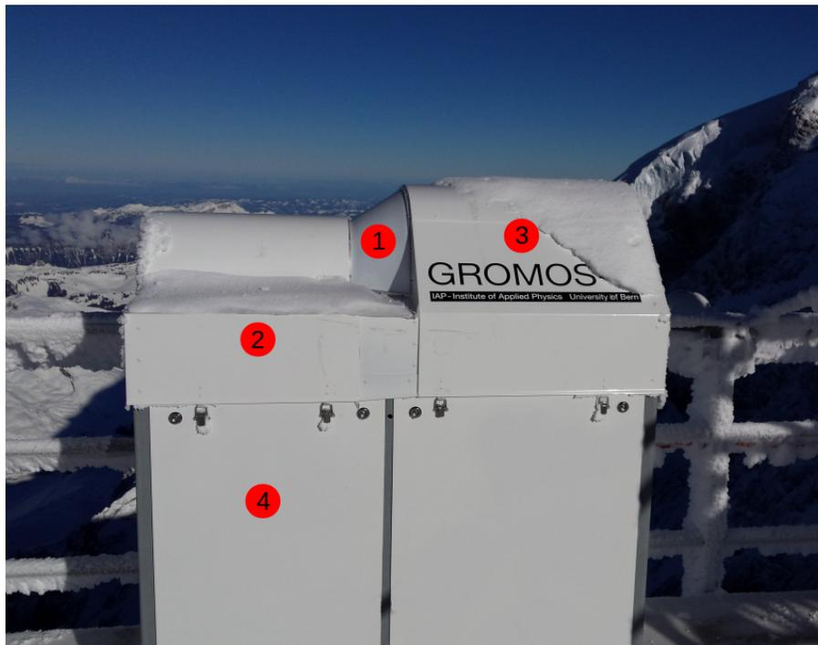
**Figure 2.** GROMOS-C at the terrace of Sphinx during the Jungfrauoch campaign. 1: Teflon window, 2: microwave receiver, 3: calibration targets, 4: computer and spectrometer.
