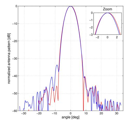
Figure 6. Planar cuts of the farfield pattern through the beam center. The blue line correponds to a scanning in elevation, and the red to a scanning in azimuth.
