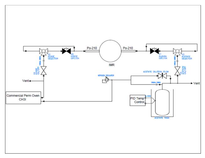
S1: Schematic diagram showing the setup for reagent switching with selectable flow path for automatic switching driven by solenoid valves or manual control.
