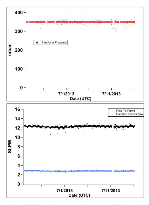
S3: Diagnostic inlet performance showing the pressure stability, the total flow through the gas sampling line, and the total flow to the pump during SOAS.
