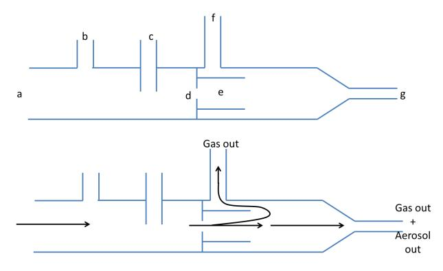
S2: Glass inlet design (a) aerosol and gas inlet; (b) zero air overflow port; (c) calibration port (not used in this study); (d) critical orifice; (e) glass particle skimmer and flow director; (f) gas sampling port at reduced pressure; (g) bypass line at reduced pressure
