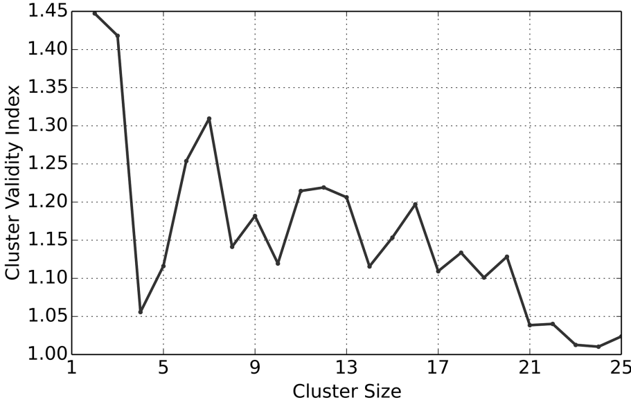
Figure 7. Application of the heuristic elbow method to identify the optimal number of clusters in which the grid cells of the studied domain of Rochor can be grouped. The drastic decrease of the clustering index with four clusters suggests that additional clusters will not significantly improve the clustering quality.
